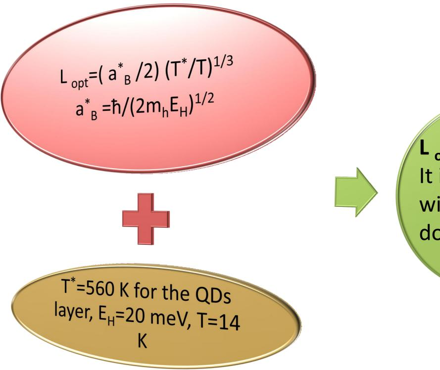
L<sub>opt</sub>=26.8nm It is comparable with the inter dots distance I. One dimensional aligned GeSi QDs along 1D trenches have been prepared.
