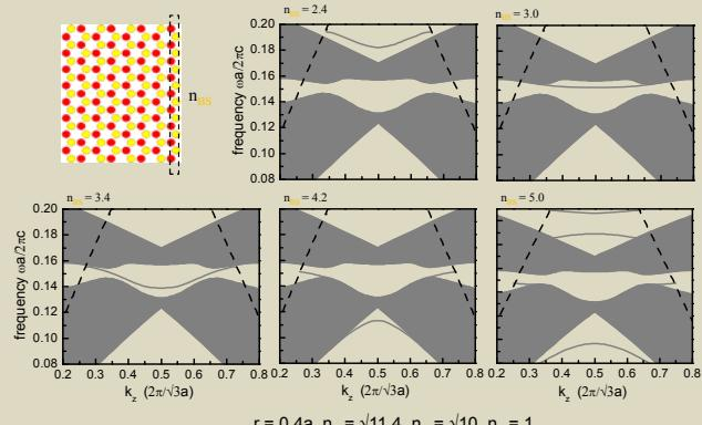
The edge states near  $k_z = \pi/\sqrt{3}a$  are almost completely localized on the outmost rods while those near the two Dirac points are much more spread into the bulk.
