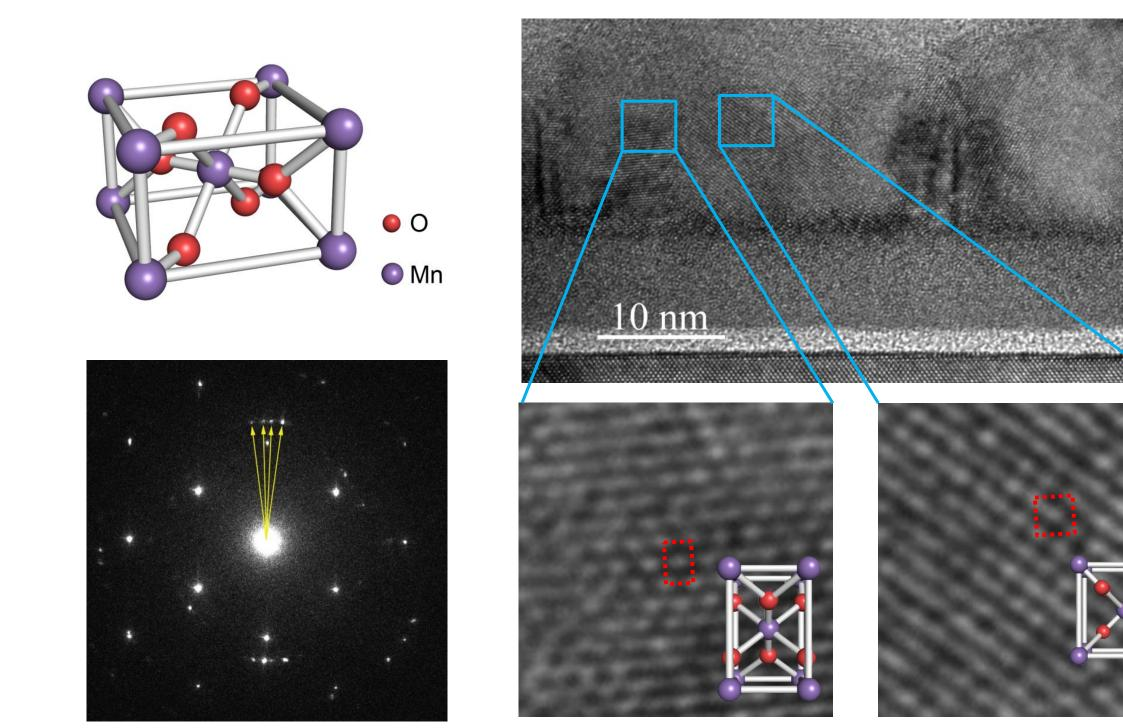
The atomic structure of the Mn oxide film was confirmed to be beta- $MnO_2$  by XRD and TEM experiments.
