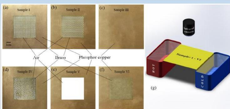
Fig. 1 Six samples illustrating the concept of quasi-uniform heat conduction.
