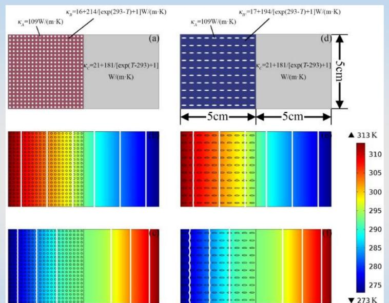
Fig. 3 Simulation results of illusion thermal diode.
