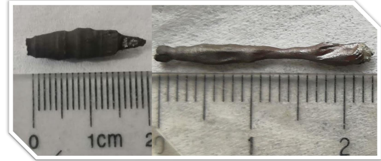
Figure 3 | Rod Crystals Obtained by Czochralski Method.
