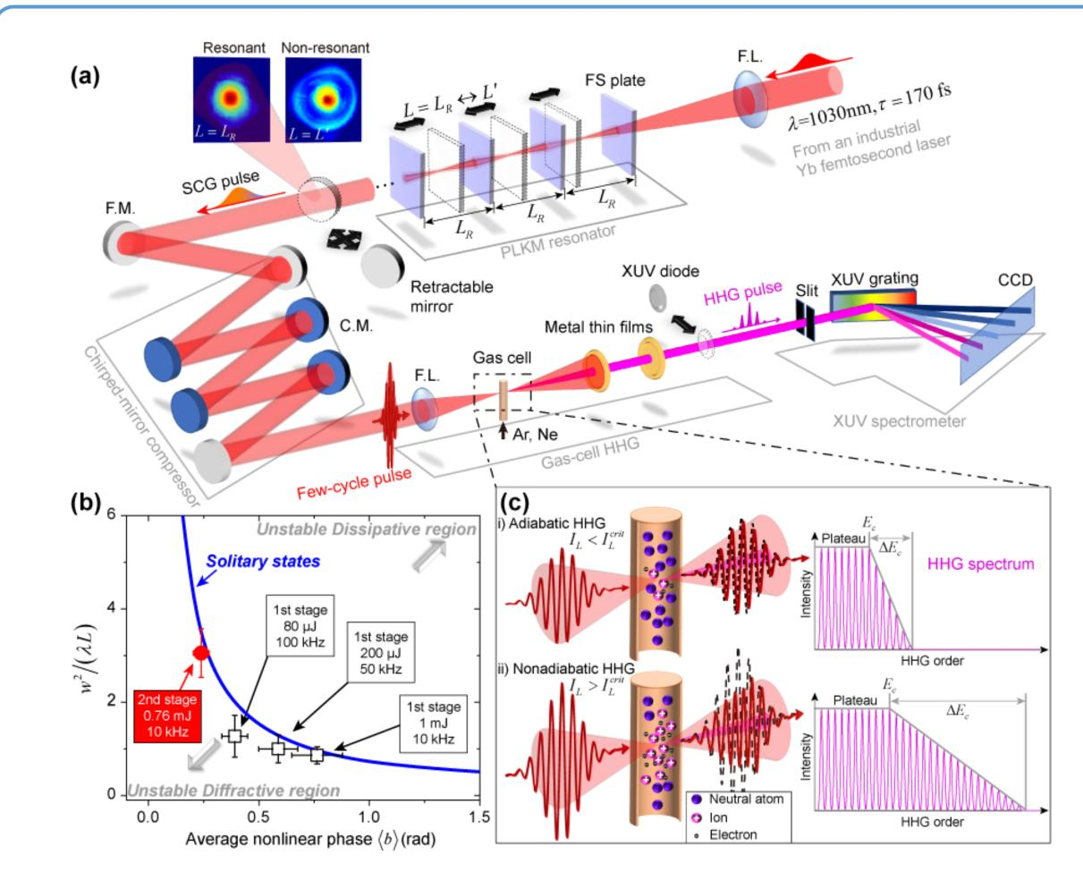
Universal relationship of the normalized beam radius squared as a function of the nonlinear phase b for the resonator solitary modes.
