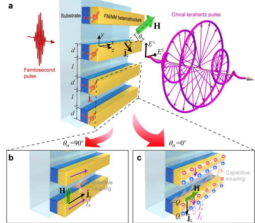
The metasurface can influence the device functionality by inducing strong amplitude and phase modulations onto the emitted terahertz waveforms.
