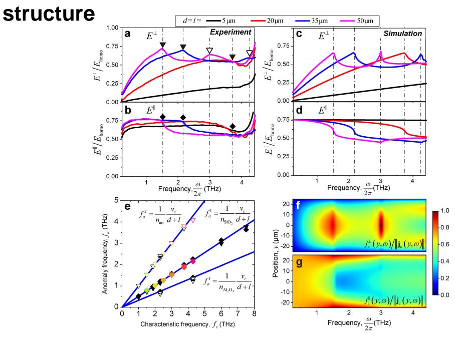
This observation confirms that the spatial confinement on the laser-induced transient currents in the stripe-patterned metasurface is responsible for the observed spectral and phase modulations, as well as for the generation of chiral terahertz waveforms.
