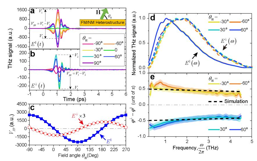
The directions parallel and perpendicular to the stripes define a set of canonical coordinates, in which the terahertz waveforms of  $E^{\parallel}$  and  $E^{\perp}$  are decoupled from each other and possess a broadband quarter-wave phase difference.
