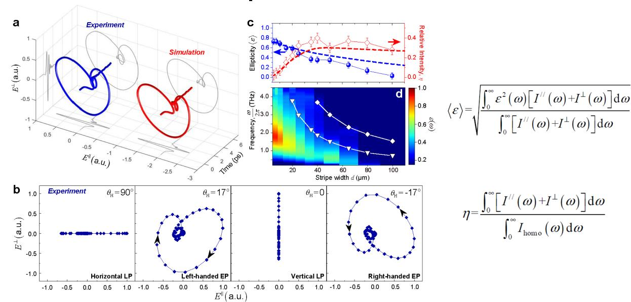
The ellipticity and handedness of the emitted terahertz radiation can be conveniently and continuously controlled by changing the field angle  $\theta_H$  because the relative quartwave phase difference can be well maintained in a broad bandwidth.
