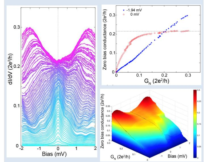
conductance of ZBCP saturates at  $0.22 \text{ G}_0(=2e^2/h)$  and side peaks exceed it that the dI/dV turns into a "gap"-like signature
