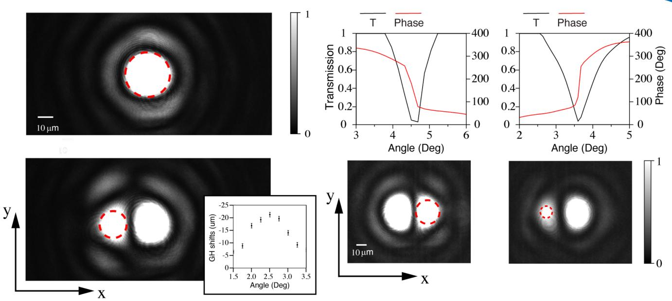
The intensity distribution of the transmitted light beam measured experimentally.
