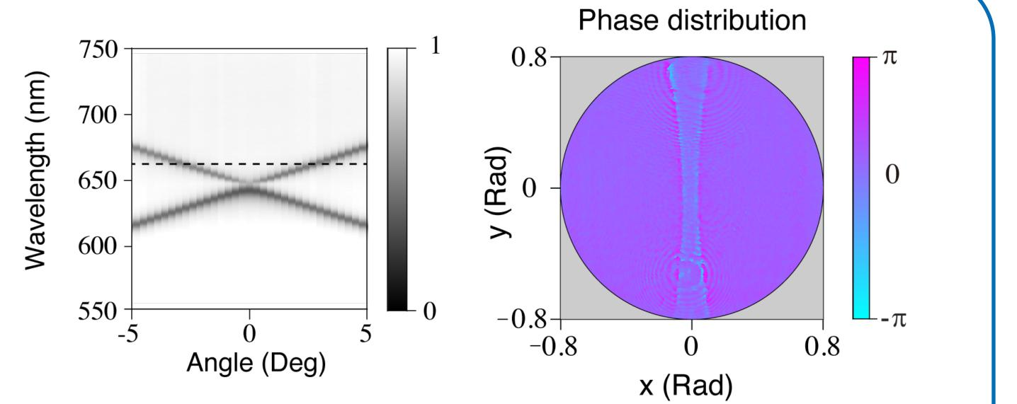
The measured angle-resolved transmittance spectra of the grating under TE-polarized incidence beam and measured phase distributions with TE- polarized incidence beam at  $\lambda = 660$  nm induced by the sample.
