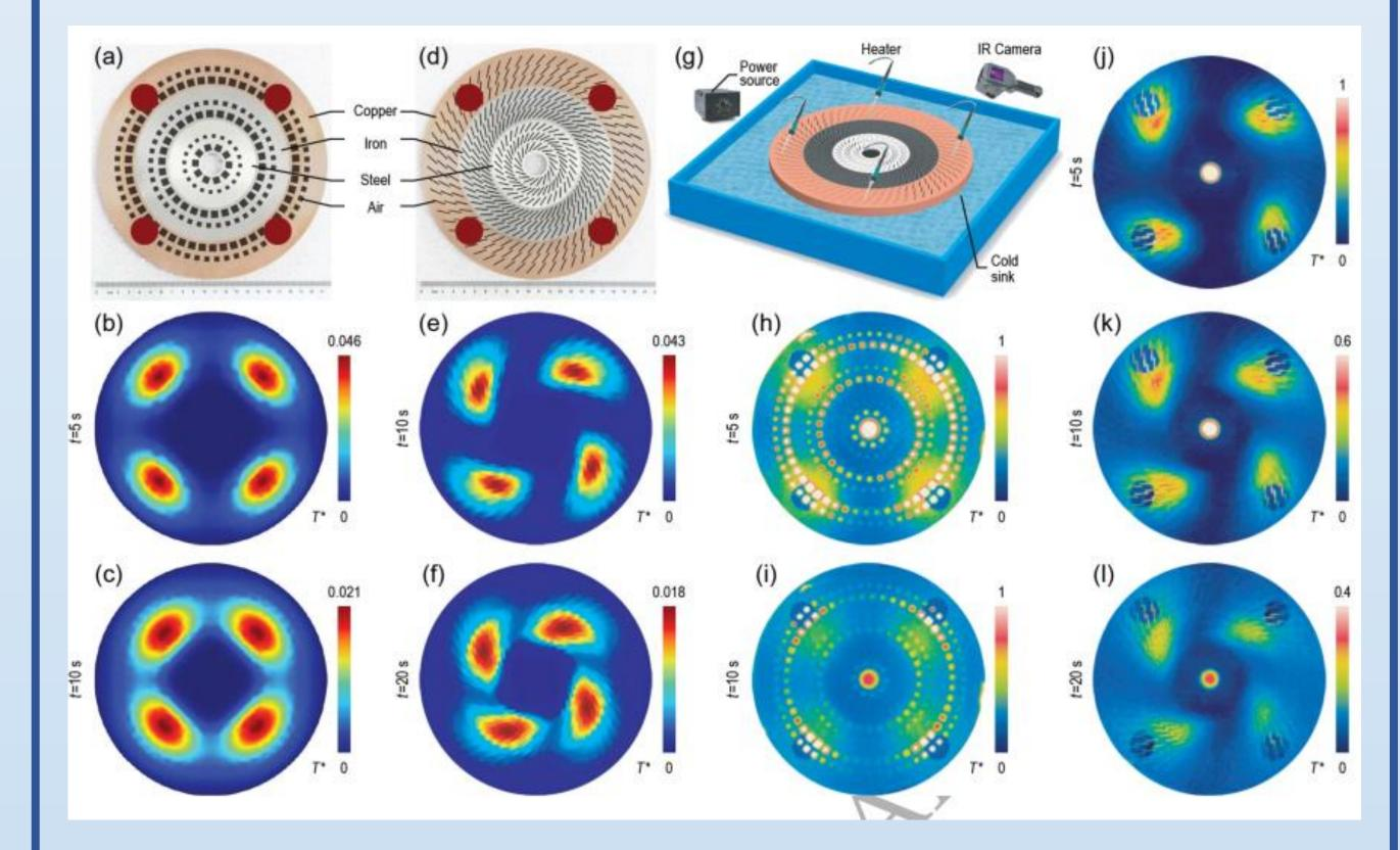
The hot spots are trapped (b and c, simulations) with the graded metadivice. Under the rotational transformation, the hot spots are trapped and rotated (e and f, simulations) with graded and anisotropic metadivice. Experiments (g-i) validate the trapping effect with time.
