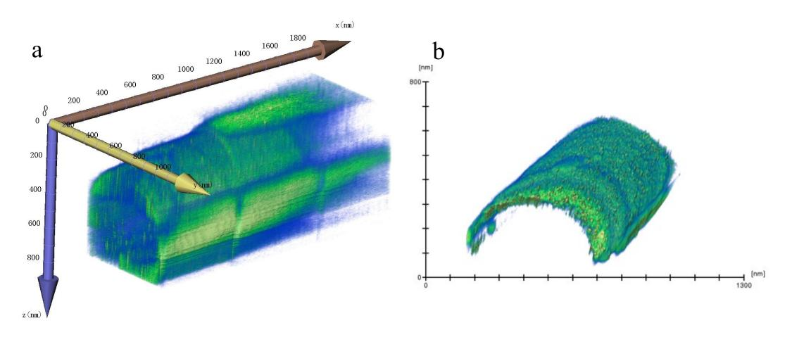
Two nanotubes coated with small crystalline nanoparticles are used as test samples. The volume render 3D image show the high spatial resolution in both the x-y direction and the z direction.
