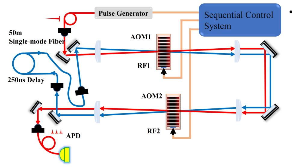
• The double-AOM drives almost all of the incoming pulse into the fiber-delayed loop (blue line), with 25% insertion loss (mainly limited by fiber loss), to be picked up on demand later.
