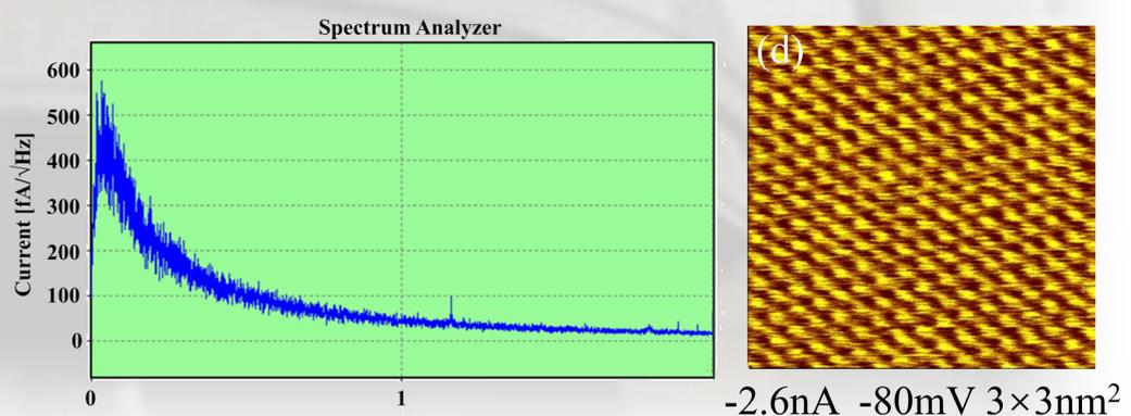
(a) Large scale STM image of HOPG surface. (b) Topography measured along redline in (a). (c) Frequency spectrum of the tunneling current at a fixed height with  $I_t=500$ pA,  $V_b=1$ V. (d) Atomic resolution STM image of HOPG.
