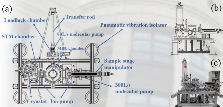
(a) Top view (b) side view of a 3D model of the system (c) photograph of the system
