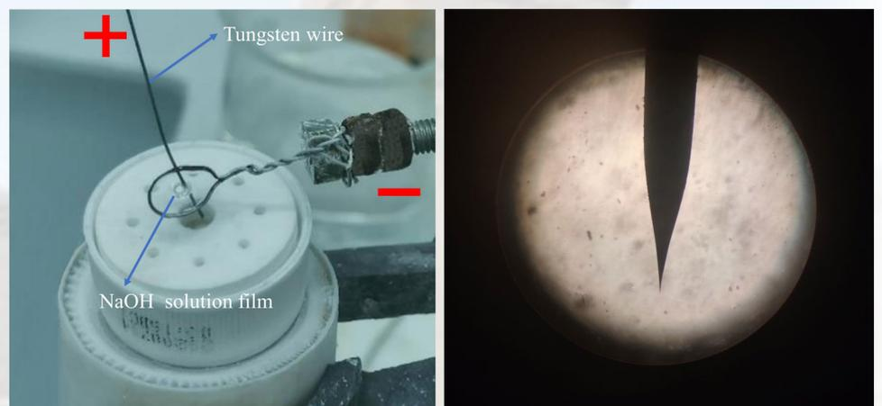
Tungsten tips are fabricated by electrochemically etching. 2 mol/L NaOH solution is chosen as electrolyte.
