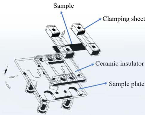
Sample is mounted between the clamping sheet and ceramic insulator for direct current heating. We chose molybdenum (Mo) as the sample holder material for better UHV compatibility and less contamination for Si-related sample.
