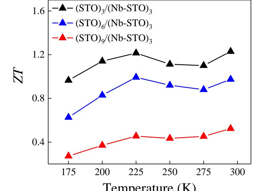
➤ Reduction of insulating layers increases the electrical conductivity and further boosts the thermoelectric performance.
