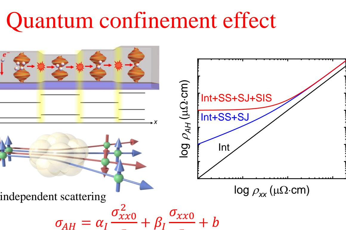
$\rho_{xx0}(\sigma_{xx0})$ : total resistivity(conductivity);  $\rho_I(\sigma_I)$ : impurity resistivity(conductivity) in bulk;  $\alpha_I$ : impurity skew scattering;  $\beta_I$ : impurity side jump
