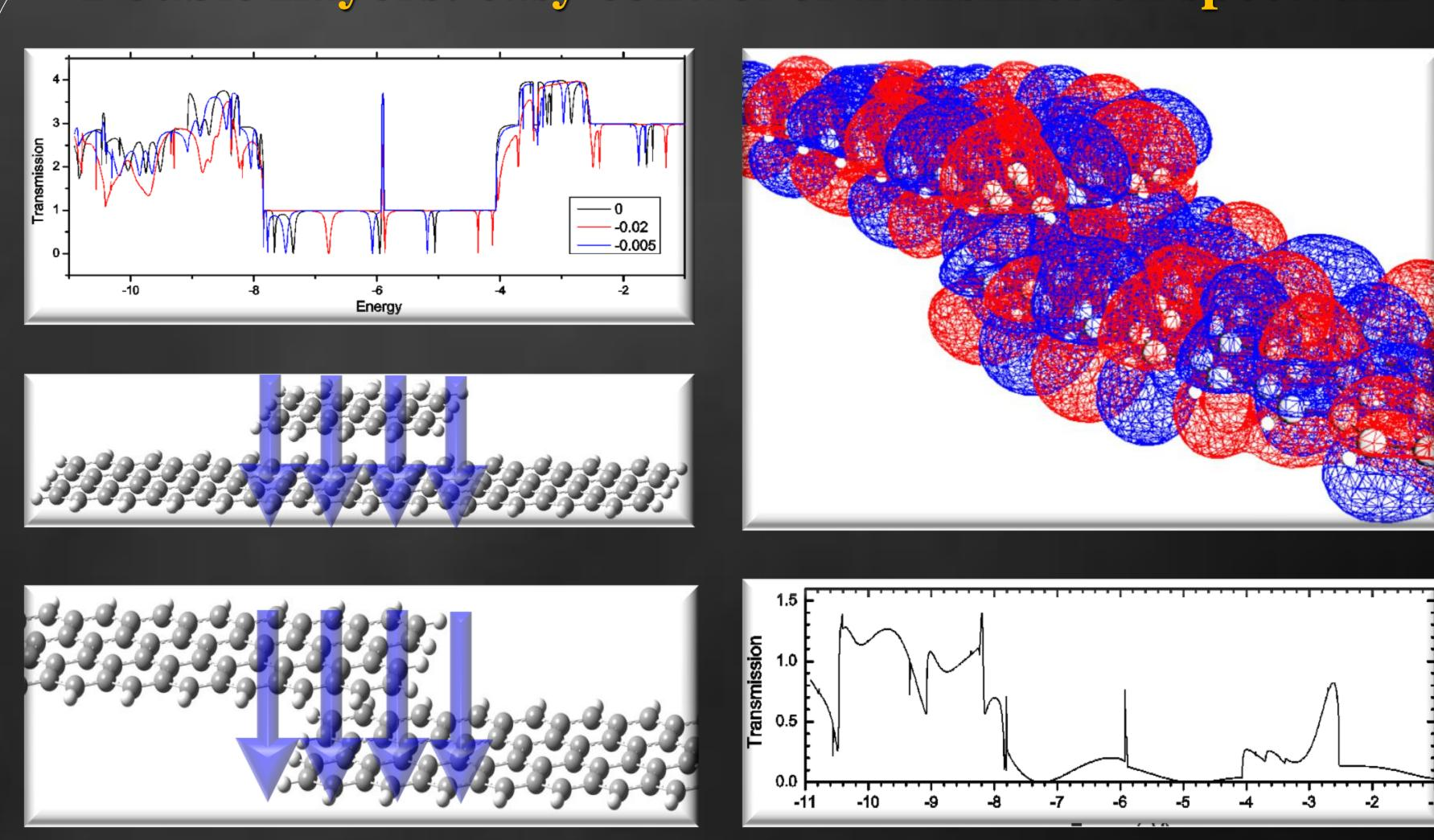
Because of strong inter-layer coupling, external field can also control the transmission of double layer devices.
