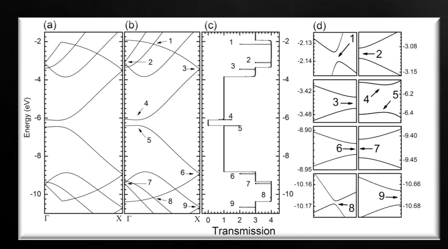
"Bad points" of step shaped transmission spectrum: mini band gaps.
