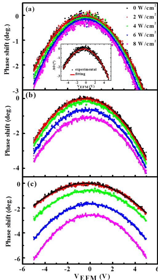
Figure 2  $\Delta\Phi - V_{EFM}$  curves measured at different laser intensities for NR1 (a), NR2 (b), and NR3 (c)..
