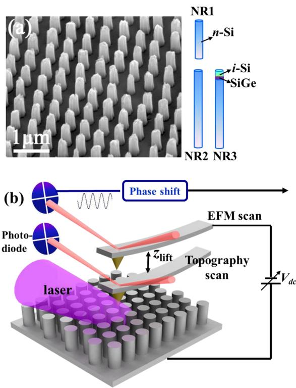
Figure 1 Constructions of NRs and schematic diagram of EFM measurements
