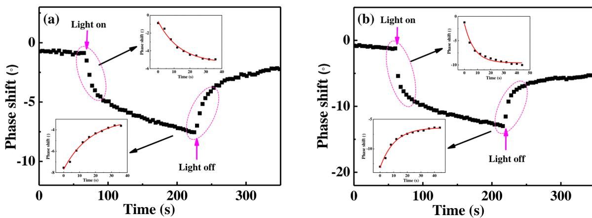
Figure 4 Time evolutions of EFM phase shift. Of NR2 (a) and NR3 (b) The exponential decay and growth fittings of the data when the laser is ON and OFF are given in the insets of the figure
