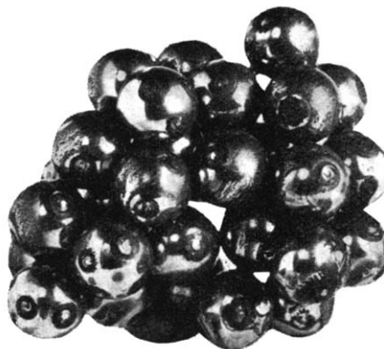
Fig. 5. Portion of random close packed ball assembly showing marks of further contacts
