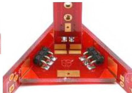
...stubby pins soldered into pads...
