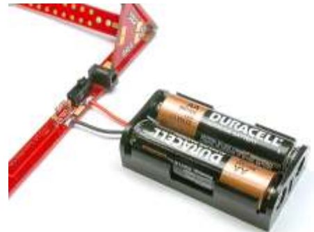
The auxiliary power pads can accommodate a battery pack or additional solar cell. A pair of AA's should last for about 2 months of continuous swinging!
