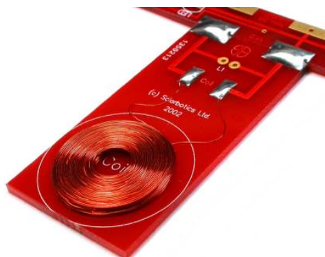
Finished coil platform installation and coil mounting
