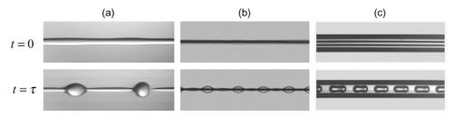
**Figure 24.** Capillary instability of cylindrical interfaces: (a) liquid jet, (b) liquid film on a fibre, (c) liquid film in a tube (adapted from [171]). The instability time  $\tau$  equals  $\sqrt{\rho h_0^3/\gamma}$  for a solid inviscid jet of radius  $h_0$ , and  $\eta h_0^4(\gamma e_0^3)$  for a thin film of thickness  $e_0$  deposited on a fibre of radius  $h_0$ .
