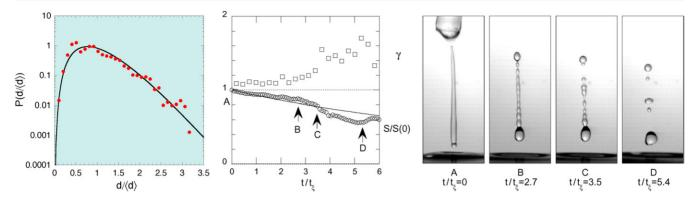
**Figure 90.** Blob size distribution of the ligament in figure 89 just prior to its breakup, fitted by a *Gamma* distribution of order n = 4.5. (Left) Evolution of the roughness  $\zeta$  of the ligament ( $\square$ ) and of the surface S/S(t=0) ( $\bullet$ ) as a function of the time in units of the capillary time  $t_{\mathcal{E}}$ . The continuous line is the prediction for S(t) based on equation (293). (Right) Corresponding ligament.
