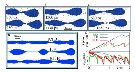
**Figure 58.** A comparison between MD simulations of the jet in figure 5 and simulations of (246) for  $M_l = 0$  (no noise, curves and profiles marked LE) and  $M_l = 0.24$  (marked SLE). From [298]. Reprinted with permission from AAAS.
