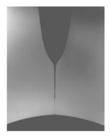
**Figure 61.** A drop of glycerol in water (85%) pinching off. Out of the main neck grow two more generations 'micro-threads' [304], which have the form of similarity solutions. From [332]. Reprinted with permission from AAAS.
