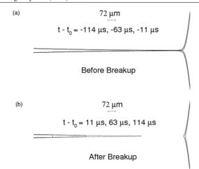
**Figure 62.** The breakup of a mixture of glycerol in four parts of ethanol, as calculated from similarity solutions before and after breakup. (a) shows three profiles before breakup, in time distances of  $46 \mu s$ , corresponding to |t'| = 1, 0.55 and 0.1. In part (b) the same is shown after breakup.
