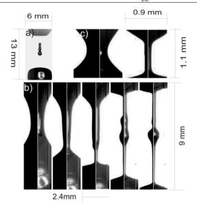
**Figure 99.** (a) A drop of water falling from a faucet,  $h_0 = 3$  mm. (b), (c): closeup of the pinch region, with 100 ppm of PEO solution added. (left: numerical simulations, right: experiment) (b):  $h_0 = 3$  mm,  $t_c - t = 6$ , 2, 0, -3, -5 ms; (c):  $h_0 = 0.4$  mm  $t_c - t = 1$ , 0 ms. Model parameters:  $\eta_p = 3.7 \times 10^{-4}$  Pa s,  $\lambda_p = 1.2 \times 10^{-2}$  s,  $b = 2.5 \times 10^4$ ,  $\eta_s = 1 \times 10^{-3}$  Pa s,  $\gamma = 6 \times 10^{-2}$  N m<sup>-1</sup>.
