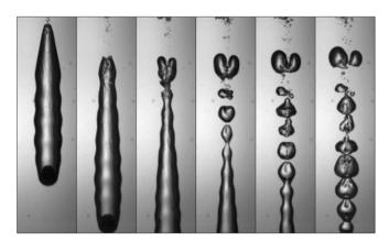
**Figure 85.** Ripple-induced breakup of the entrained bubble behind a 1/2 in. diameter steel sphere impacting at 4.1 m s<sup>-1</sup> in water. Courtesy of A Belmonte [477]. Reprinted with permission, copyright 2007 by the American Physical Society.
