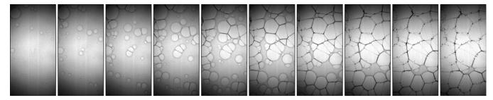
**Figure 83.** Bursting of a soap film accelerated by the parallel impact of a shock wave. Time goes from left to right with time step  $\Delta t = 0.05$  ms. Incoming wave Mach number is M = 1.21 [471].
