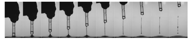
**Figure 28.** A pipette dipping into still water is rapidly removed vertically, producing a liquid ligament from the elongation of the bridge between the liquid and the pipette end. When the motion is fast enough, the ligament stretches while remaining smooth. As soon as the stretching stops, because the ligament is no longer connected to the liquid bath, it breaks into drops.
