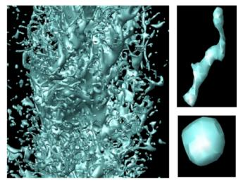
**Figure 35.** The intricate forest of liquid ligaments and drops in a flow similar to that of figure 34 revealed by numerical simulations [78]. Courtesy of A Berlemont.
