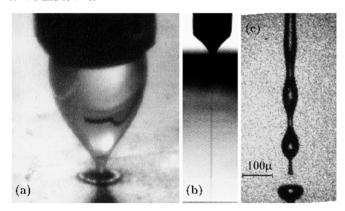
**Figure 67.** A view of the experimental apparatus. Fluid is sucked through a hole opposite a capillary tube (a). This leads to a much thinner micro-jet (b). This micro-jet decays into droplets by surface tension forces (c). Reprinted with permission from [379]. Copyright 1998 by the American Physical Society.
