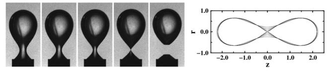
**Figure 55.** (Left) The pinch-off of an air bubble in water [326]. An initially smooth shape develops a localized pinch point. (Right) Numerical simulation of bubble pinch-off from initial conditions given by the shape with the largest waist; there is no gravity, so all shapes are symmetric about the pinch point. Reprinted with permission from [326], copyright 2007 by the American Physical Society.
