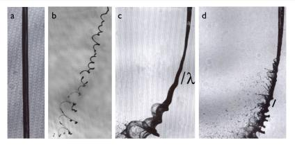
**Figure 46.** Liquid jet in a transverse cross flow of air. (a) Reference jet with no air, (b) We = 3, (c) We = 8, (d) We = 30 with  $We = \rho_a u^2 d/\gamma$  as defined in (171). The jet diameter is millimetric and the liquid velocity  $v_0$  is of the order of a few  $10 \,\mathrm{m\,s^{-1}}$ . The bar indicates the length of the Rayleigh–Taylor wavelength  $\lambda$ . Courtesy of K A Sallam [277].
