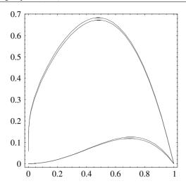
**Figure 20.** A comparison between dispersion relations  $-\omega^2(k)\tau^2$  for inviscid flow, as function of  $kh_0$ . There is excellent agreement between the exact formula (57) for a fluid jet and the long-wavelength form (62) (top curves), as well as the analogous formulae for a hollow jet (equations (69) and (77), bottom curves).
