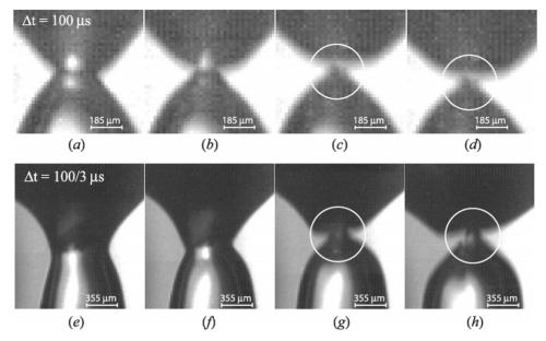
**Figure 57.** A fast gas jet blowing through an inertial liquid. The bubble pinches off extremely violently. Adapted from [297], with permission. Original figure copyright 2005 by the American Physical Society.
