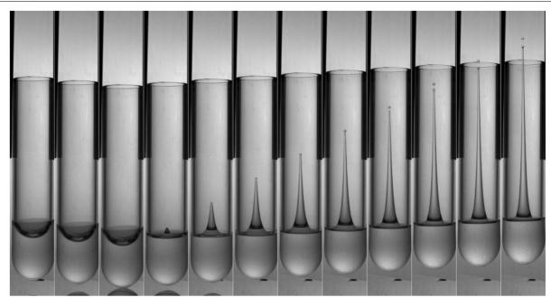
**Figure 73.** Axial impact of a cylindrical tube falling under gravity and filled with a liquid wetting the tube wall. Following the impact on a rigid floor, the curvature of the spherical meniscus initially fixed by the tube radius reverses violently, a prelude to the birth of a rapidly ascending jet [426].
