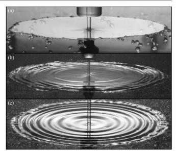
**Figure 77.** Axisymmetric liquid sheet states: (*a*) Smooth regime. (*b*) Flapping regime for larger Weber number (higher than 1000). (*c*) Perturbation of the smooth regime by imposing vertical oscillations of the impact rod. Adapted from [278].
