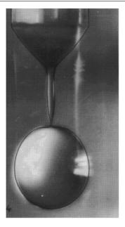
**Figure 14.** The shape of a drop of water falling from a nozzle at the first bifurcation [28]; the parameters are Bo = 1.02 and  $Oh = 2.2 \times 10^{-3}$ . The line is the result of a boundary integral computation [53]. Reprinted with permission from Cambridge University Press.
