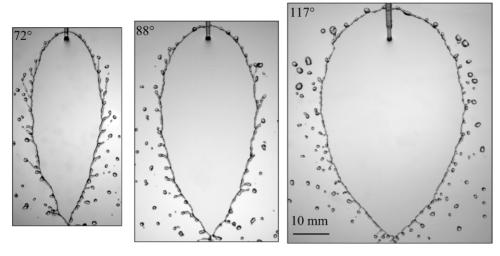
Figure 79. Water sheet fragmentation for three collision angles, the jet velocity is equal to  $4 \,\mathrm{m\,s^{-1}}$  and the jet diameter is 1.05 mm. Elongation of ligaments is clearly enhanced when the collision angle is decreased [456].
