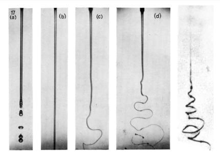
**Figure 42.** (Left) Whipping instability. Water jet exposed to an increasing longitudinal potential difference from left to right [244]. (Right) Strobe photograph of the overall picture of an unstable jet. Reprinted with permission from [247], copyright 2001 by the American Institute of Physics.
