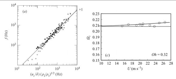
Figure 39. (Left) Passage frequency f of the optimal disturbance of the interface as a function of frequency, compared with the prediction of (140). Here  $u_c$  stands for the group velocity in (138). Measurements are from [232,235]. (Right) Dimensionless growth rates  $\Omega_i = \omega \tau$  of perturbations growing on a liquid jet issuing into air as a function of the jet speed U. The wavelength is close to the optimum value. Experimental data are from [148], theory according to [236].
