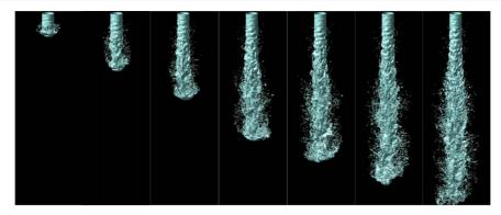
**Figure 17.** A numerical simulation of a turbulent jet of liquid ( $\rho_{liq} = 696 \, kg \, m^{-3}$ ,  $\eta_{liq} = 1.2 \times 10^{-3} \, kg \, (ms)^{-1}$ ) entering a gas atmosphere ( $\rho_{gas} = 25 \, kg \, m^{-3}$ ,  $\eta_{gas} = 10^{-5} \, kg \, (ms)^{-1}$ ) [78]. The surface tension is  $\gamma = 0.06 \, N \, m^{-1}$ , the jet speed is  $v_{nozzle} = 100 \, m \, s^{-1}$ , the turbulence intensity [79] is 0.05.
