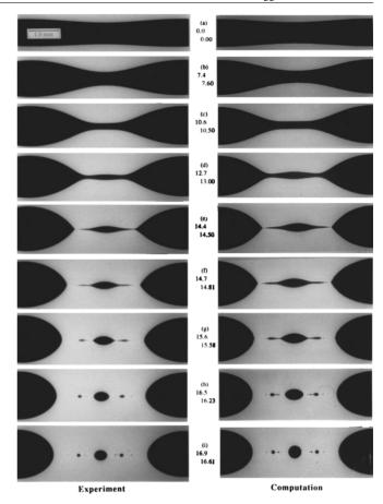
**Figure 15.** Time evolution of a cylinder of fluid suspended in another fluid. The viscosity ratio is  $\lambda = 0.0067$ , and the initial dimensionless wavenumber x = 0.5 [57]. Snapshots are taken at the times shown in the middle. Reprinted with permission from Cambridge University Press.
