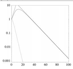
**Figure 29.** Temporal evolution of the amplitude  $\epsilon(t)/\epsilon(0)$  according to equation (103) for  $\sigma=0.2$  (weak stretching, continuous line) and  $\sigma=0.8$  (strong stretching, dashed line), with  $kh_0=1/\sqrt{2}$ . The straight lines are the short time growth, and long-time relaxation limit behaviours for  $\sigma=0.2$ . Time t is in units of  $\sigma^{-1}$ .
