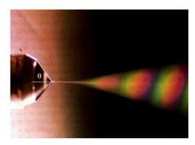
**Figure 64.** A Taylor cone in the cone-jet mode (reprinted from [365], copyright 1994, with permission from Elsevier). The opening half-angle shown is  $\theta = 52^{\circ}$ . A large voltage difference is maintained between the capillary on the left, and an electrode on the right. The cone-like structure on the right is produced by a cloud of little droplets.
