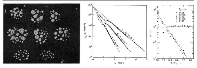
Figure 75. (Left) Raindrop specimens [30] captured by allowing drops to fall into a 1 in. deep layer of fine un-compacted flour. (Middle) drop size distributions for three different rainfall rates [436]. (Right) Cumulative drop size distribution  $\eta = \int_{R}^{\infty} p(R, R_0) dR$  resulting from the breakup of a drop with initial radius  $R_0$  falling in air [439].
