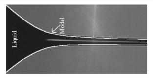
**Figure 65.** Comparison between theory, based on the slender-jet description (253), (255) and experiment with an ethylene glycol jet at  $Q = 2.78 \times 10^{-9} \,\mathrm{m}^3 \,\mathrm{s}^{-1}$ . Reprinted from [371], copyright 1999, with permission from Elsevier.
