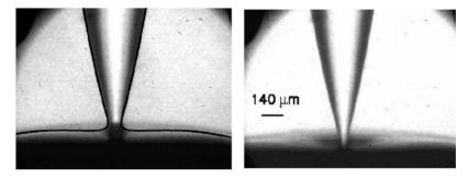
Figure 52. Closeup of the pinching of a water drop [74]. The left picture is a comparison with a full Navier–Stokes simulation, the right picture is taken at an angle to show overturning. Reprinted with permission from [74]. Copyright 2002 by the American Physical Society.
