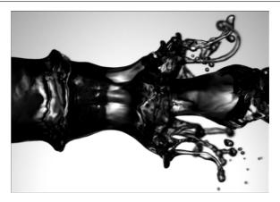
**Figure 38.** Destabilization of a slow water jet ( $h_0 \approx 4$  mm) by a fast coaxial air stream [232] ( $v_1 = 0.6 \,\mathrm{m\,s^{-1}}, \, v_2 = 35 \,\mathrm{m\,s^{-1}}$ ). The wavelength of the primary axisymmetric undulation is governed by (137).
