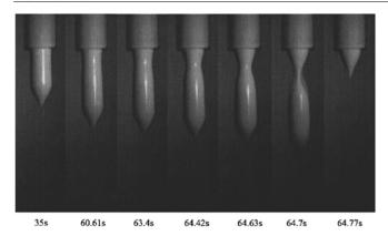
**Figure 101.** Successive views of a mayonnaise sample at different times, pushed out of a nozzle of radius  $h_0 = 3$  mm. The initial time (0 s) corresponds to the separation of the previous extrudate. Reprinted with permission from [523]. Copyright 2005 by the American Physical Society.
