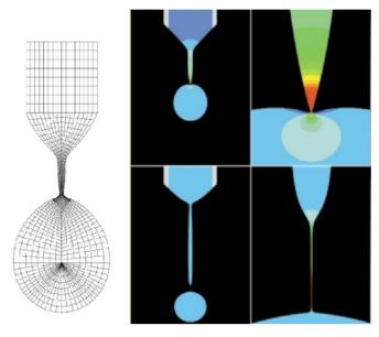
**Figure 16.** Schematic of tessellation (left), and simulations of dripping (right). The nozzle radius is R = 3.6 mm, the top picture corresponds to water, the bottom to a 83% glycerol solution. Reprinted from [73]. Copyright 2002, with permission of John Wiley and Sons.
