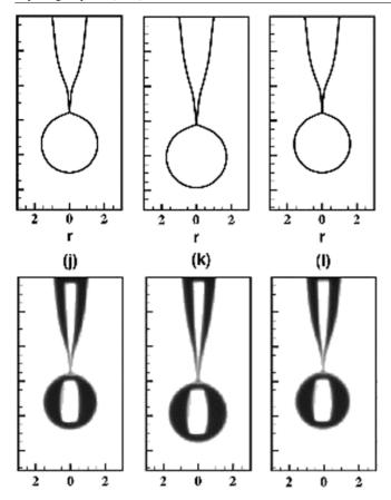
**Figure 18.** Period-2 dripping at Oh = 0.13, Bo = 0.33, and We = 0.232 [97]. (Top) simulation of (29),(30), (bottom) experiment. Reprinted with permission from [97], copyright 2006 by the American Institute of Physics.
