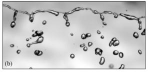
**Figure 78.** Close-up views of the free rim of a smooth liquid sheet, taken from the top (a). In (b), a periodic vibration of the impact point at 120 Hz has been added. The scale indicated in (a) is the same for both images, and  $h_0 = 3$  mm. Adapted from [278].
