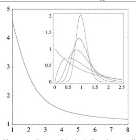
**Figure 92.** Average diameter of the drop's dispersion normalized by the ligament initial average radius  $\langle d \rangle / \xi$ , as a function of n according to (297) for N(0) = 125. An initially strongly corrugated ligament gives rise to an average droplet size appreciably larger than its average initial diameter. Inset: corresponding distributions  $p(d/\langle d \rangle)$  as a function of  $d/\langle d \rangle$  for n = 1, 2, 5, 10, 25.
