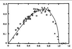
**Figure 19.** Dimensionless growth rate  $-i\omega(k)\tau$  of sinusoidal perturbations on a cylinder as a function of the dimensionless wave number  $kh_0$ . The solid line represents Rayleigh's theory for inviscid flow [120, 159]. Reprinted with permission from [159], copyright 1975 by the American Institute of Physics.
