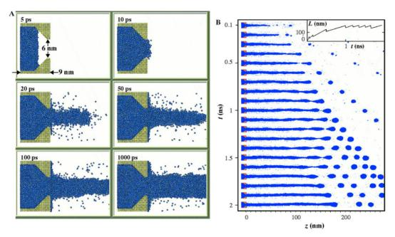
**Figure 5.** A MD simulation of a jet of propane coming out of a gold nozzle 6 nm in diameter (see section 4.5, figure 58). From [298]. Reprinted with permission from AAAS.
