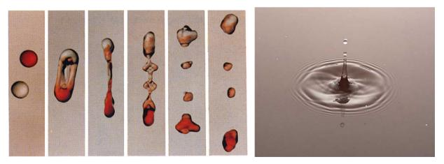
Figure 72. (Left) Binary collision of drops, stretching and fragmentation. We = 83 based on the relative velocity between the drops [420]. Reprinted with permission from Cambridge University Press. (Right) A jet emerging from the closing cavity left after the impact of a drop on a layer of the same liquid.
