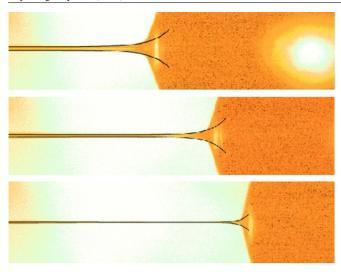
**Figure 49.** A sequence of interface profiles of a jet of glycerol close to the point of breakup [304] (the centre of the drop being formed is seen as a bright spot in the top picture). The experimental images correspond to  $t_0 - t = 350$ , 298 and 46  $\mu$ s (from top to bottom). Corresponding analytical solutions based on (200), (201) are superimposed [120]. There is no adjustable parameter in the comparison.
