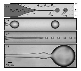
**Figure 27.** A coflowing liquid stream, driven by the outer fluid [179]. (a) device geometry, (b) dripping regime, (c) jetting, kepping the inner flow rate  $q_{\rm in}$  constant, but increasing  $q_{\rm out}$ ;  $\eta_{\rm in}/\eta_{\rm out}=0.1$ . (d) widening jet, obtained by increasing  $q_{\rm in}$ . Reprinted with permission from [179]. Copyright 2007 by the American Physical Society.
