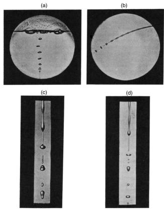
**Figure 9.** Plate I of Rayleigh's 'some applications of photography' (1891) [23] showing the destabilization of a jet of air into water (a) of a water jet in air (b). Rayleigh notes that the air jet destabilizes faster than the water jet. Details of the breakup process and the recoil of initially straight 'ligaments' between the drops, sometimes breaking themselves before they have recoiled (c) and (d).
