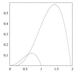
**Figure 41.** Stability curve  $-i\omega\tau$  versus  $kh_0$ . Destabilizing effect of surface charges with  $\Gamma=2$  on the varicose mode m=0 in equation (150). The neutral jet dispersion curve is shown for comparison.
