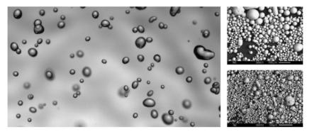
Figure 69. (Left) Drops in a liquid spray formed in an uncontrolled way are naturally distributed in size. (Right) Solid tin powder formed from the atomization of a liquid tin stream for two operating conditions [392]. Obviously the resulting powder is far from uniform in size.
