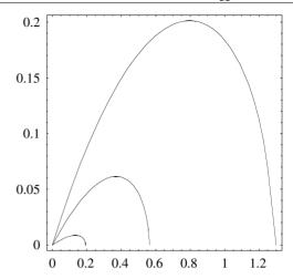
**Figure 36.** Dispersion relation Re[ $-i\omega_i(k)$ ] as given by (136), shown as a function of  $k\delta$  for three different density ratios  $\rho_a/\rho = 1, 0.1, 0.01$ .
