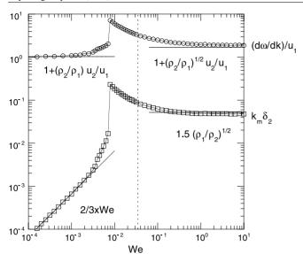
**Figure 37.** Transition from a thin shear layer to a thick shear layer as a function of the Weber number  $We_{\delta}$  for  $v_2/v_1 = 20$ , using the parameters of an air/water interface;  $\bigcirc$ , group velocity;  $\square$ , most unstable wavenumber; - - - -, transition value of  $(\rho_2/\rho_1)^{1/2}$ .
