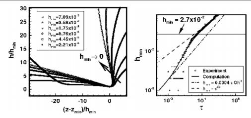
**Figure 51.** (Left) Profiles from a Navier–Stokes simulation of the pinch-off of a water drop ( $Oh = 1.81 \times 10^{-3}$ ), the axes are rescaled by  $h_{\min}$ . (Right)  $h_{\min}/r_0$  for a 83% glycerol–water mixture ( $Oh = 1.63 \times 10^{-1}$ ), showing crossover from the Euler to the Navier–Stokes solution. Reprinted with permission from [74]. Copyright 2002 by the American Physical Society.
