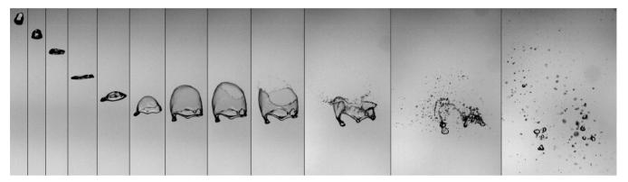
**Figure 76.** Fragmentation of a water drop (diameter 5 mm) falling in an ascending stream of air [404]. Images are taken at (t = 0, 4, 9, 17, 24, 30, 33, 34, 35, 37, 43 and 60 ms.)
