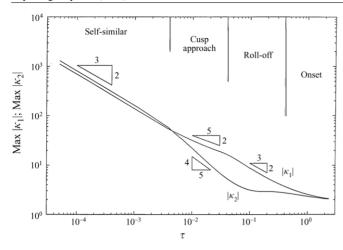
**Figure 88.** Time sequence of the maximum principal curvatures of a liquid bridge as it pinches-off under mild stretching (see also figure 87). Time  $\tau = t_p - t$  is the time from pinch-off. The onset of the instability, as well the boundary conditions influence the evolutions down to  $10^{-2}-10^{-3}$  of the overall time  $t_p$ , after which the dynamics is universal. Adapted from [289].
