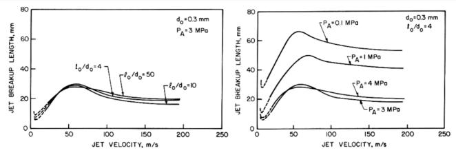
Figure 47. Liquid intact lengths (or jet breakup length) measured for increasing jet velocity  $v_0$  for various injection conditions ( $d_0$  is the injector diameter and  $\ell_0$  denotes the orifice length, setting the boundary layer thickness at the exit) as well as different ambient gas pressures. (Adapted from Hiroyasu *et al* (1982) [282]).
