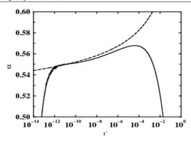
**Figure 56.** A comparison of the exponent  $\alpha$  between full numerical simulations of bubble pinch-off (——) and the leading-order asymptotic theory (239) (- - - -).
