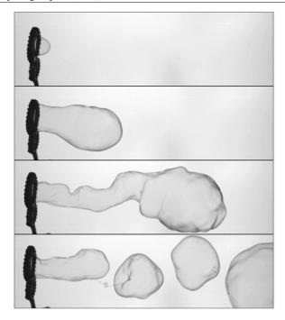
**Figure 21.** Blowing on a soap film inflates it in the form of a hollow tube which destabilizes into a train of soap bubbles. The wavelength is consistently given by the tube radius.
