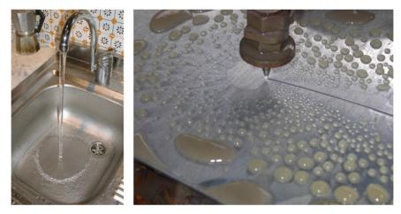
**Figure 2.** (Left) A jet of tap water falling into a sink. The jet is too thick and its falling time too short for breakup to occur, yet it has become rough. The continuous jet hits the sink floor, where it expands radially in the form of a thin sheet boarded by a hydraulic jump. (Right) Higher speed water jets are also used to cut tissues, meat, and even metal plates.
