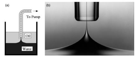
**Figure 68.** In the selective withdrawal experiment, two viscous liquids are layered atop of one another. The upper, more viscous liquid is withdrawn through a capillary and entrains a thin stream of the lower liquid. From [380]. Reprinted with permission from AAAS.
