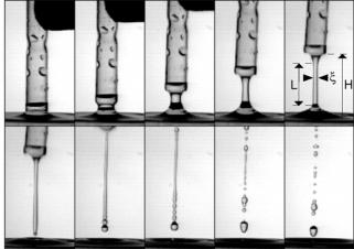
**Figure 87.** Condition for ligament formation from the withdrawal of a capillary tube (diameter D=7 mm) whose end dips into water [510]. (Left) Ligament contraction with a slow tube elevation velocity (time intervals  $\Delta t=10.7$  ms). (Right) Fast elongation and ligament formation ( $\Delta t=4.5$  ms).
