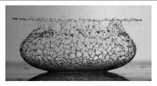
**Figure 81.** The 'crystal crown' formed by the impact of a 5 mm viscous drop (89% glycerin/water solution) onto a 35  $\mu$ m thick layer of ethanol (We = 5720). Marangoni forces thin the sheet locally, leading to a myriad of holes, ligaments and then drops [469]. Reprinted with permission from Cambridge University Press.
