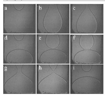
**Figure 50.** Nine images (of width 3.5 mm) showing how a  $^{3}$ He crystal 'flows' down from the upper part of a cryogenic cell into its lower part [308]. The recording takes a few minutes, the temperature is approximately 0.32 K. The crystal first 'drips' down, so that a crystalline 'drop' forms at the bottom (a)–(c); then a second drop appears (d) and comes into contact with the first one (e); coalescence is observed (f) and subsequently breakup occurs (h).
