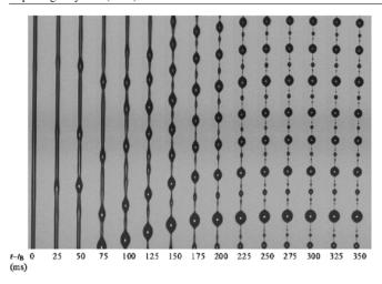
**Figure 100.** Blistering of an aqueous solution of  $M_{\rm w}=3.8\times10^6\,{\rm g\,cm^{-3}}$  PEO solution at a concentration of  $c=2000\,{\rm ppm}$ . Reprinted with permission from [515], copyright 2005 by the American Institute of Physics.
