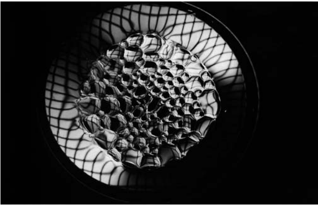
Fig. 13. Rose window fully developed in an ohmic liquid (castor oil) in a triode set-up. The instability is stationary even at voltages higher than the critical value. V_p=12 kV, V_g=3.25 kV, I=1.55 \mu A, p=3.0 cm, h=1.5 cm, d=1.2 mm
