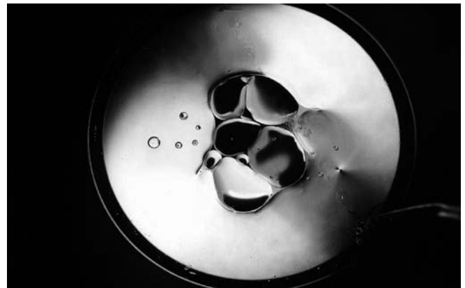
Fig. 12. The non-homogeneity of the electric field is greater in a tip-plane configuration. The first incipient instability appears at the centre of the electrode. Liquid: castor oil. V_p=6.8 kV, I=0.404 \mu A, L=3.1 cm, p=3.0 cm, d=1.2 mm
