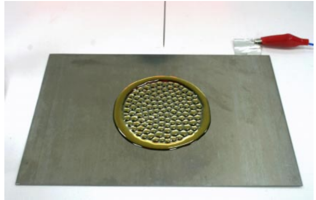
Figure 2. A drop of oil in the field of corona discharge.
