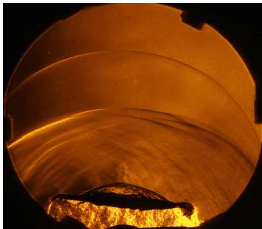
Fig. 9. A pulsed schlieren image displays external shock waves beyond the end of the tube (Ref. 1). The convergence of shock waves (centered vertically) has served to remove the tape, and the singular shock wave in the upper half of the image is an earlier shock wave partially reflected internally back toward the ball. Hot air pulses out behind the tape, and the ball is just starting to emerge at the bottom.
