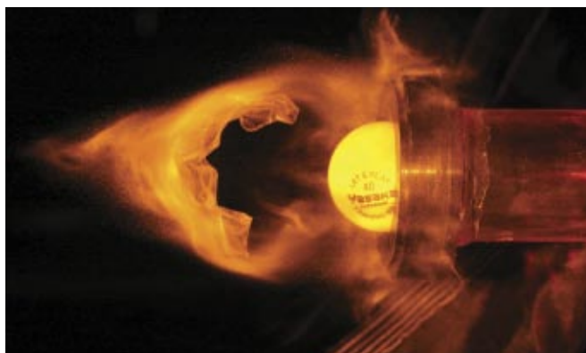
Fig. 3. Laser pulse of 0.4\ \mu\text{s} images the ball following the tape upon exit from the 3.6-m acrylic tube.
