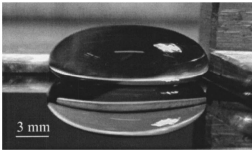
FIG. 2. Large water droplet deposited on a silicon surface at 200 °C.
