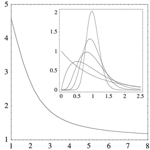
**Figure 92.** Average diameter of the drop's dispersion normalized by the ligament initial average radius  $\langle d \rangle / \xi$ , as a function of  $n$  according to (297) for  $N(0) = 125$ . An initially strongly corrugated ligament gives rise to an average droplet size appreciably larger than its average initial diameter. Inset: corresponding distributions  $p(d/\langle d \rangle)$  as a function of  $d/\langle d \rangle$  for  $n = 1, 2, 5, 10, 25$ .
