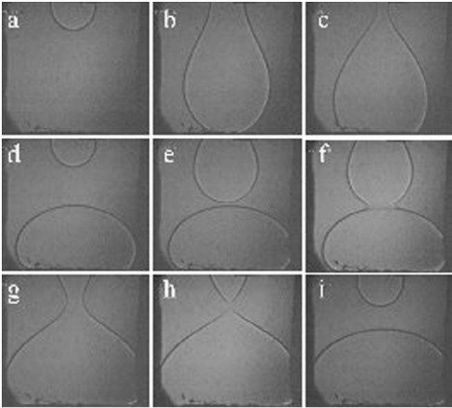
**Figure 50.** Nine images (of width 3.5 mm) showing how a  $^3\text{He}$  crystal ‘flows’ down from the upper part of a cryogenic cell into its lower part [308]. The recording takes a few minutes, the temperature is approximately 0.32 K. The crystal first ‘drips’ down, so that a crystalline ‘drop’ forms at the bottom (a)–(c); then a second drop appears (d) and comes into contact with the first one (e); coalescence is observed (f) and subsequently breakup occurs (h).
