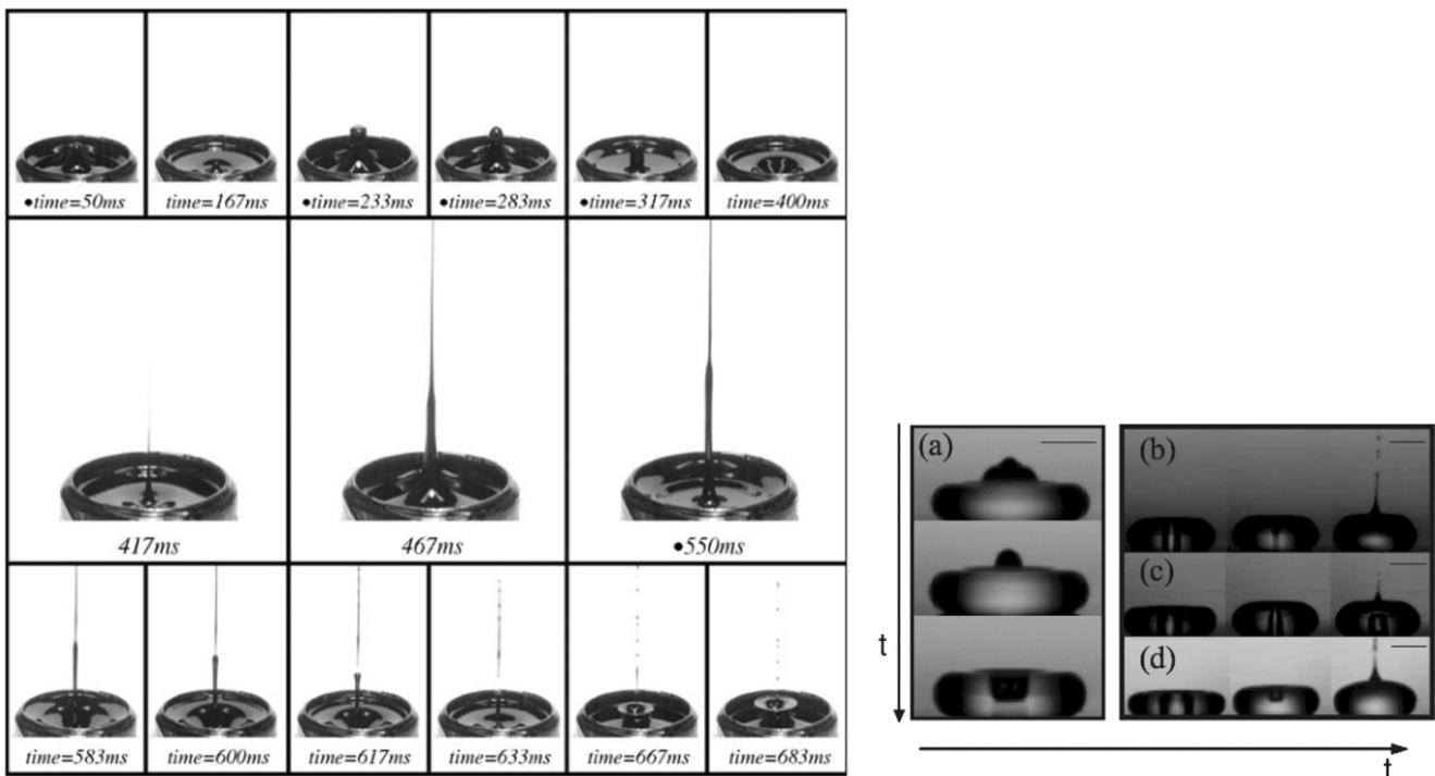
**Figure 74.** (Left) Sequence of frames showing a rapidly moving jet evolving from an over-forced standing wave in a ferrofluid [427]. (Right) Impact of a (millimetric) water drop on a super-hydrophobic surface, formation of a cavity and ejection of a highly focused jet. Reprinted with permission from [428]. Copyright 2006 by the American Physical Society.
