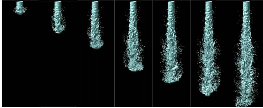
**Figure 17.** A numerical simulation of a turbulent jet of liquid ( $\rho_{\text{liq}} = 696 \text{ kg m}^{-3}$ ,  $\eta_{\text{liq}} = 1.2 \times 10^{-3} \text{ kg (ms)}^{-1}$ ) entering a gas atmosphere ( $\rho_{\text{gas}} = 25 \text{ kg m}^{-3}$ ,  $\eta_{\text{gas}} = 10^{-5} \text{ kg (ms)}^{-1}$ ) [78]. The surface tension is  $\gamma = 0.06 \text{ N m}^{-1}$ , the jet speed is  $v_{\text{nozzle}} = 100 \text{ m s}^{-1}$ , the turbulence intensity [79] is 0.05.
