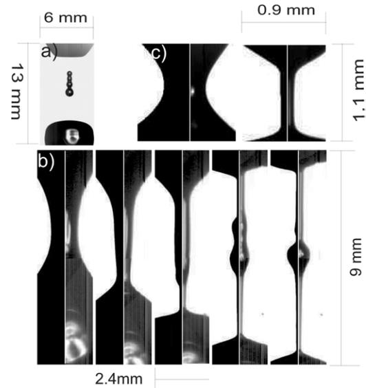
**Figure 99.** (a) A drop of water falling from a faucet,  $h_0 = 3$  mm. (b), (c): closeup of the pinch region, with 100 ppm of PEO solution added. (left: numerical simulations, right: experiment) (b):  $h_0 = 3$  mm,  $t_c - t = 6, 2, 0, -3, -5$  ms; (c):  $h_0 = 0.4$  mm  $t_c - t = 1, 0$  ms. Model parameters:  $\eta_p = 3.7 \times 10^{-4}$  Pa s,  $\lambda_p = 1.2 \times 10^{-2}$  s,  $b = 2.5 \times 10^4$ ,  $\eta_s = 1 \times 10^{-3}$  Pa s,  $\gamma = 6 \times 10^{-2}$  N m $^{-1}$ .
