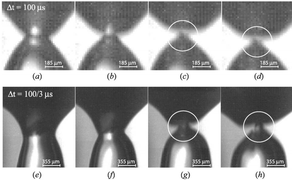
**Figure 57.** A fast gas jet blowing through an inertial liquid. The bubble pinches off extremely violently. Adapted from [297], with permission. Original figure copyright 2005 by the American Physical Society.
