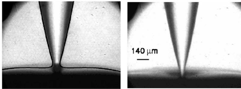
**Figure 52.** Closeup of the pinching of a water drop [74]. The left picture is a comparison with a full Navier–Stokes simulation, the right picture is taken at an angle to show overturning. Reprinted with permission from [74]. Copyright 2002 by the American Physical Society.
