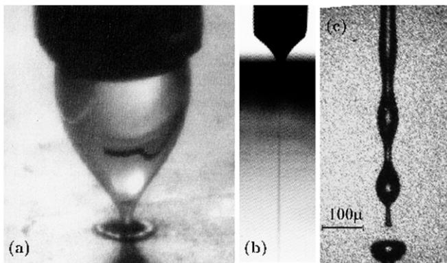
**Figure 67.** A view of the experimental apparatus. Fluid is sucked through a hole opposite a capillary tube (a). This leads to a much thinner micro-jet (b). This micro-jet decays into droplets by surface tension forces (c). Reprinted with permission from [379]. Copyright 1998 by the American Physical Society.
