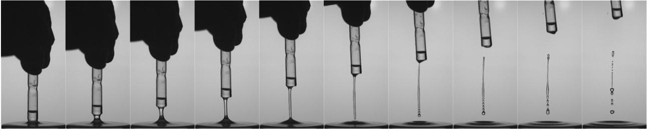
**Figure 28.** A pipette dipping into still water is rapidly removed vertically, producing a liquid ligament from the elongation of the bridge between the liquid and the pipette end. When the motion is fast enough, the ligament stretches while remaining smooth. As soon as the stretching stops, because the ligament is no longer connected to the liquid bath, it breaks into drops.
