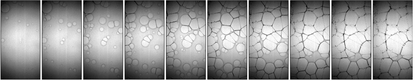
**Figure 83.** Bursting of a soap film accelerated by the parallel impact of a shock wave. Time goes from left to right with time step  $\Delta t = 0.05$  ms. Incoming wave Mach number is  $M = 1.21$  [471].
