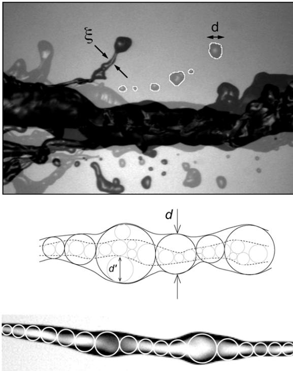
**Figure 89.** Double flash exposure of a ligament torn off by the wind (section 5.1) just before and after breakup. (Middle) A sketch of the layer interaction scheme. (Bottom) An isolated ligament covered with blobs of various sizes  $d$  corresponding to the local thickness.
