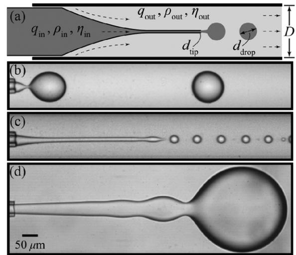
**Figure 27.** A coflowing liquid stream, driven by the outer fluid [179]. (a) device geometry, (b) dripping regime, (c) jetting, keeping the inner flow rate  $q_{\text{in}}$  constant, but increasing  $q_{\text{out}}$ ;  $\eta_{\text{in}}/\eta_{\text{out}} = 0.1$ . (d) widening jet, obtained by increasing  $q_{\text{in}}$ . Reprinted with permission from [179]. Copyright 2007 by the American Physical Society.
