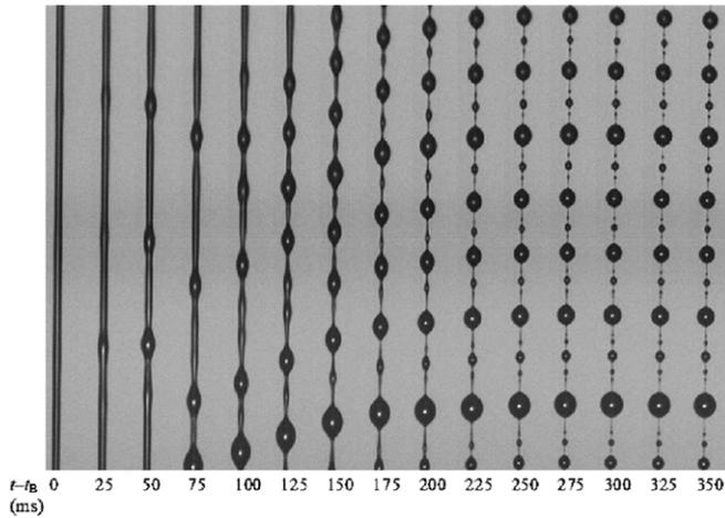
**Figure 100.** Blistering of an aqueous solution of  $M_w = 3.8 \times 10^6 \text{ g cm}^{-3}$  PEO solution at a concentration of  $c = 2000 \text{ ppm}$ . Reprinted with permission from [515], copyright 2005 by the American Institute of Physics.
