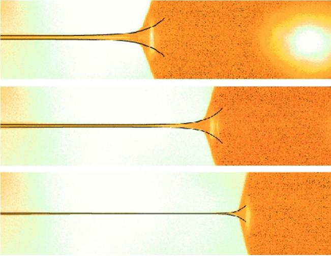
**Figure 49.** A sequence of interface profiles of a jet of glycerol close to the point of breakup [304] (the centre of the drop being formed is seen as a bright spot in the top picture). The experimental images correspond to  $t_0 - t = 350, 298$  and  $46 \mu\text{s}$  (from top to bottom). Corresponding analytical solutions based on (200), (201) are superimposed [120]. There is no adjustable parameter in the comparison.
