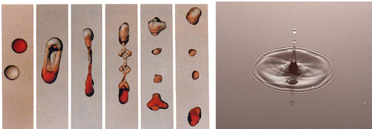
**Figure 72.** (Left) Binary collision of drops, stretching and fragmentation.  $We = 83$  based on the relative velocity between the drops [420]. Reprinted with permission from Cambridge University Press. (Right) A jet emerging from the closing cavity left after the impact of a drop on a layer of the same liquid.
