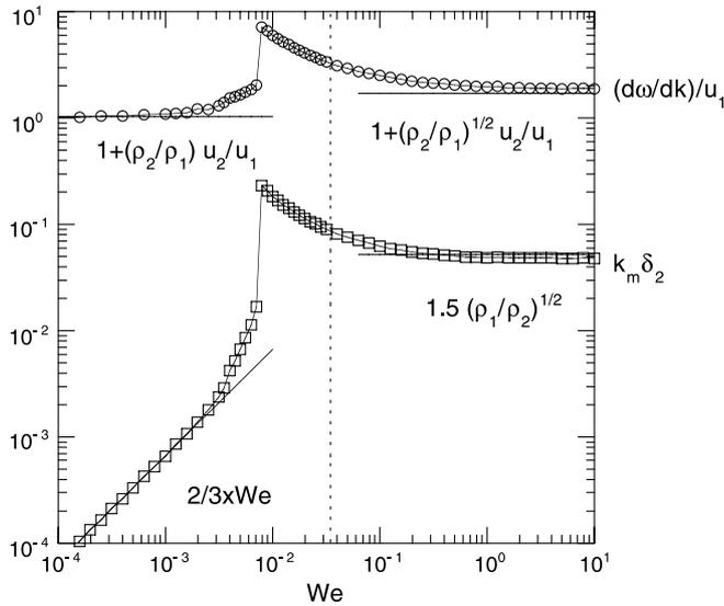
**Figure 37.** Transition from a thin shear layer to a thick shear layer as a function of the Weber number  $We_\delta$  for  $v_2/v_1 = 20$ , using the parameters of an air/water interface;  $\circ$ , group velocity;  $\square$ , most unstable wavenumber; - - -, transition value of  $(\rho_2/\rho_1)^{1/2}$ .
