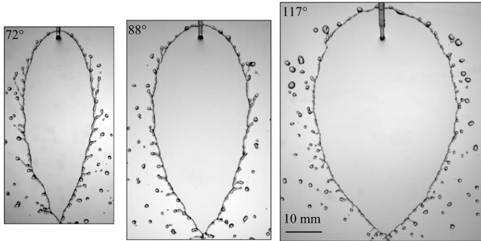
**Figure 79.** Water sheet fragmentation for three collision angles, the jet velocity is equal to  $4 \text{ m s}^{-1}$  and the jet diameter is  $1.05 \text{ mm}$ . Elongation of ligaments is clearly enhanced when the collision angle is decreased [456].
