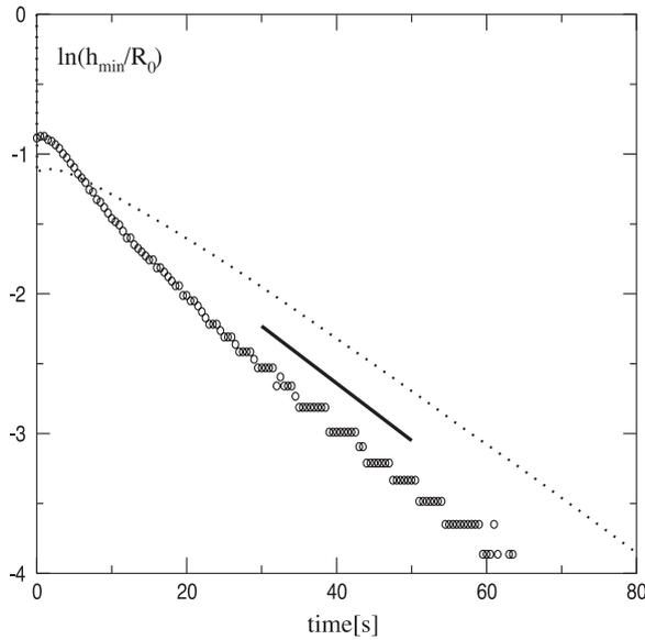
**Figure 98.** The logarithm of the normalized minimum radius of a liquid bridge, which was produced by a very rapid initial stretch [316]. The circles correspond to experiment, theory to the dotted line. The thick line is the theoretical prediction for the slope  $-1/(3\lambda)$ .
