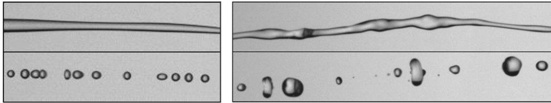
**Figure 91.** An initially smooth ligament produces a set of close to mono-disperse drops, while a rough ligament breaks into drops with a broad collection of sizes. The parameter  $n$  is large on the left and small on the right.
