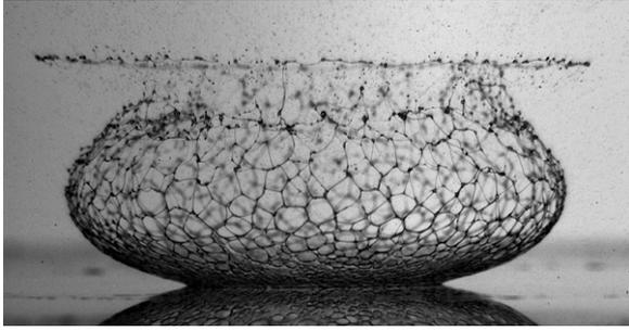
**Figure 81.** The ‘crystal crown’ formed by the impact of a 5 mm viscous drop (89% glycerin/water solution) onto a 35  $\mu\text{m}$  thick layer of ethanol ( $We = 5720$ ). Marangoni forces thin the sheet locally, leading to a myriad of holes, ligaments and then drops [469]. Reprinted with permission from Cambridge University Press.
