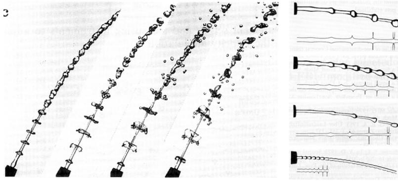
**Figure 32.** Kinematic gatherings (shocks) formed by a pulsatile axial velocity at the jet exit  $v(z=0, \tau) = v_0(1 + \epsilon \sin(\omega\tau))$ . Pure kinematics anticipates that the jet's cross-section blows up in finite time, i.e. at a finite distance from the exit. Surface tension bounds the blow-up forming a finite extent radial sheet. (Adapted from [210].)
