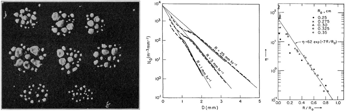
**Figure 75.** (Left) Raindrop specimens [30] captured by allowing drops to fall into a 1 in. deep layer of fine un-compacted flour. (Middle) drop size distributions for three different rainfall rates [436]. (Right) Cumulative drop size distribution  $\eta = \int_R^\infty p(R, R_0) dR$  resulting from the breakup of a drop with initial radius  $R_0$  falling in air [439].
