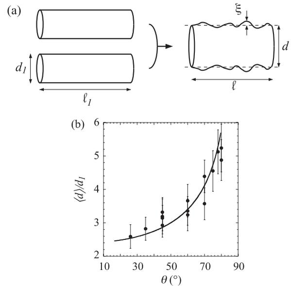
**Figure 95.** (a) Schematic of jet merging, and surface roughness generation. Corrugations expanded in Fourier modes:  $\xi = \sum_k \epsilon_k \cos(kx)$ . (b) Dependence of the average drop size from the destabilization of the resulting jet on the impact angle. Solid line is  $\langle d \rangle / d_1 = \sqrt{2} / \cos \theta$ .
