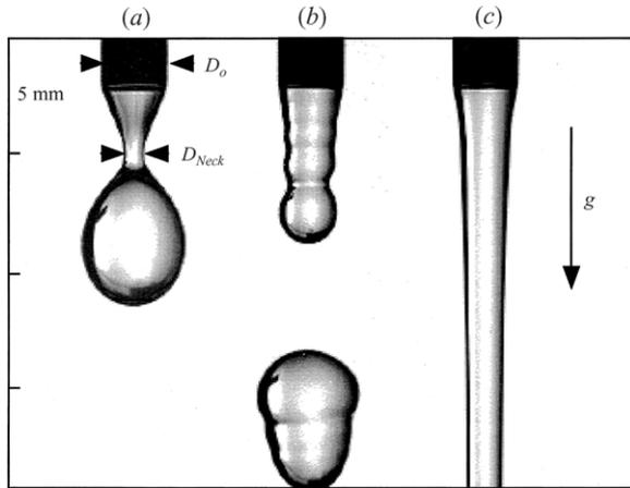
**Figure 26.** The transition from dripping to jetting for water issuing from a tube of radius  $h_0 = 1.08$  mm. (a)  $We = 0.031$  (dripping), (b)  $We = 0.86$  (chaotic dripping), (c)  $We = 1.15$  (jetting). (Adapted from [176], with permission from Cambridge University Press.)
