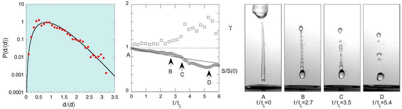
**Figure 90.** Blob size distribution of the ligament in figure 89 just prior to its breakup, fitted by a *Gamma* distribution of order  $n = 4.5$ . (Left) Evolution of the roughness  $\zeta$  of the ligament ( $\square$ ) and of the surface  $S/S(t=0)$  ( $\bullet$ ) as a function of the time in units of the capillary time  $t_\xi$ . The continuous line is the prediction for  $S(t)$  based on equation (293). (Right) Corresponding ligament.
