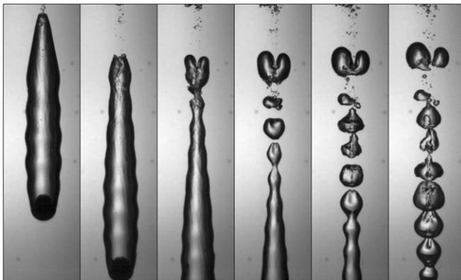
**Figure 85.** Ripple-induced breakup of the entrained bubble behind a 1/2 in. diameter steel sphere impacting at  $4.1 \text{ m s}^{-1}$  in water. Courtesy of A Belmonte [477]. Reprinted with permission, copyright 2007 by the American Physical Society.
