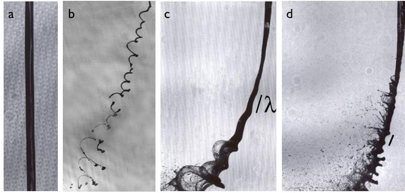
**Figure 46.** Liquid jet in a transverse cross flow of air. (a) Reference jet with no air, (b)  $We = 3$ , (c)  $We = 8$ , (d)  $We = 30$  with  $We = \rho_a u^2 d / \gamma$  as defined in (171). The jet diameter is millimetric and the liquid velocity  $v_0$  is of the order of a few  $10 \text{ m s}^{-1}$ . The bar indicates the length of the Rayleigh–Taylor wavelength  $\lambda$ . Courtesy of K A Sallam [277].
