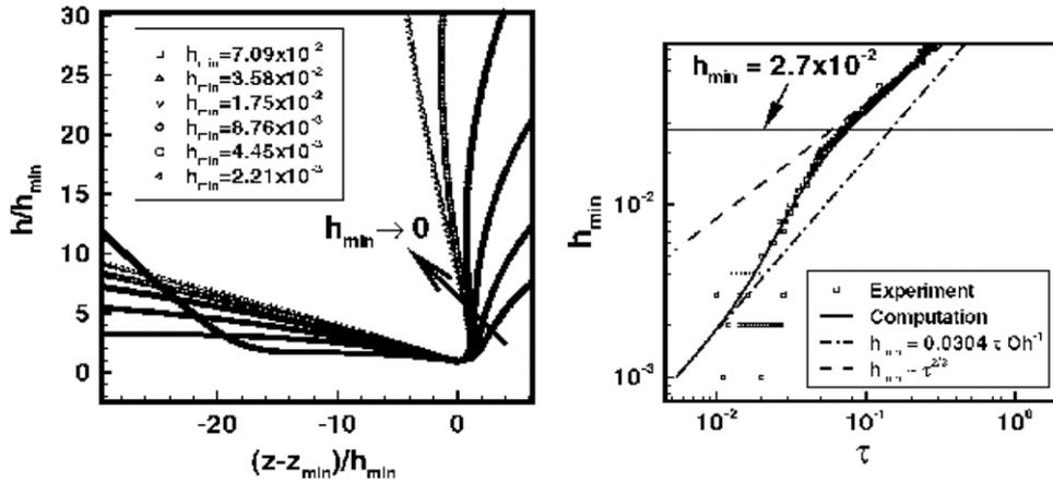
**Figure 51.** (Left) Profiles from a Navier–Stokes simulation of the pinch-off of a water drop ( $Oh = 1.81 \times 10^{-3}$ ), the axes are rescaled by  $h_{\min}$ . (Right)  $h_{\min}/r_0$  for a 83% glycerol–water mixture ( $Oh = 1.63 \times 10^{-1}$ ), showing crossover from the Euler to the Navier–Stokes solution. Reprinted with permission from [74]. Copyright 2002 by the American Physical Society.
