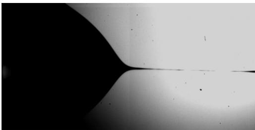
**Figure 59.** A drop of silicone oil, viscosity  $\eta = 300$  mPa, falling from a tap [334]. The width of the frame is 2 mm. Just before breakup, the thin thread has become unstable and produced several ‘bumps’. The moment of breakup shows irregular breakup at several places.
