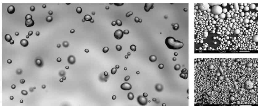
**Figure 69.** (Left) Drops in a liquid spray formed in an uncontrolled way are naturally distributed in size. (Right) Solid tin powder formed from the atomization of a liquid tin stream for two operating conditions [392]. Obviously the resulting powder is far from uniform in size.
