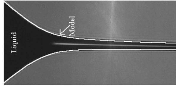
**Figure 65.** Comparison between theory, based on the slender-jet description (253), (255) and experiment with an ethylene glycol jet at  $Q = 2.78 \times 10^{-9} \text{ m}^3 \text{ s}^{-1}$ . Reprinted from [371], copyright 1999, with permission from Elsevier.
