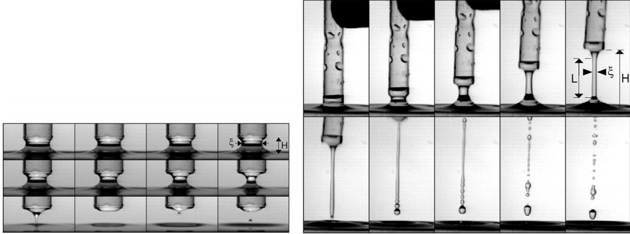
**Figure 87.** Condition for ligament formation from the withdrawal of a capillary tube (diameter  $D = 7$  mm) whose end dips into water [510]. (Left) Ligament contraction with a slow tube elevation velocity (time intervals  $\Delta t = 10.7$  ms). (Right) Fast elongation and ligament formation ( $\Delta t = 4.5$  ms).
