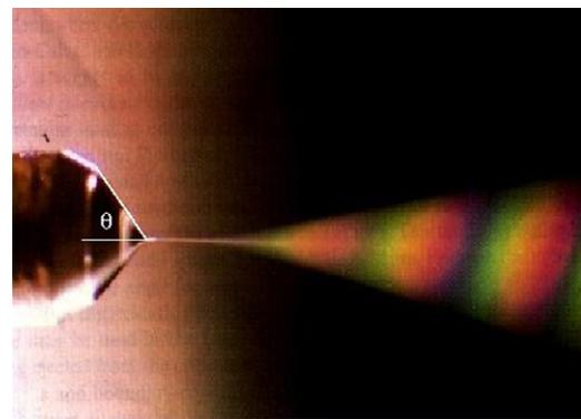
**Figure 64.** A Taylor cone in the cone-jet mode (reprinted from [365], copyright 1994, with permission from Elsevier). The opening half-angle shown is  $\theta = 52^\circ$ . A large voltage difference is maintained between the capillary on the left, and an electrode on the right. The cone-like structure on the right is produced by a cloud of little droplets.
