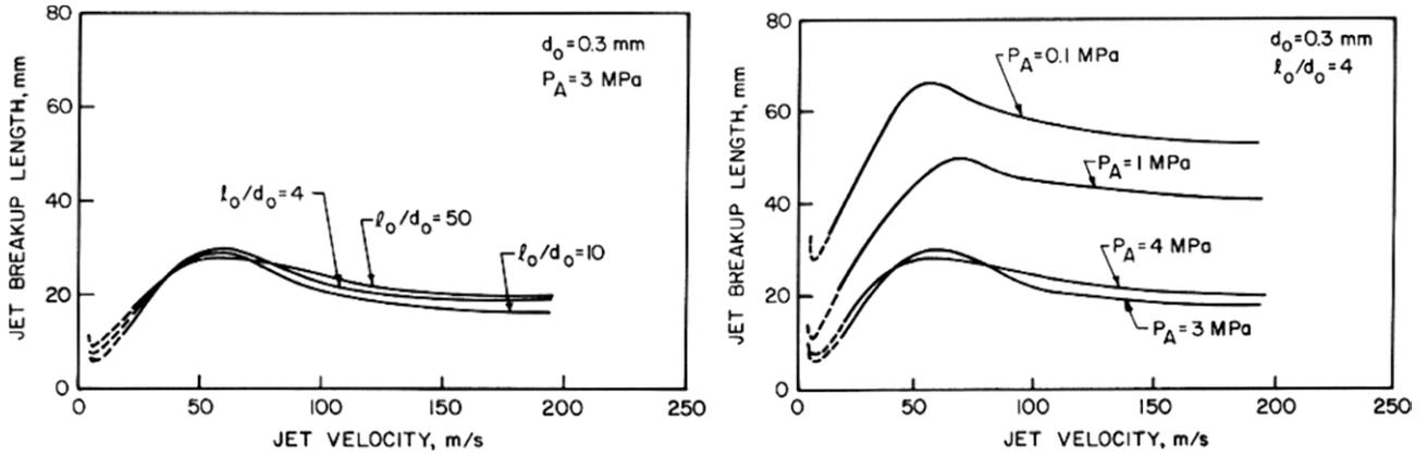
**Figure 47.** Liquid intact lengths (or jet breakup length) measured for increasing jet velocity  $v_0$  for various injection conditions ( $d_0$  is the injector diameter and  $\ell_0$  denotes the orifice length, setting the boundary layer thickness at the exit) as well as different ambient gas pressures. (Adapted from Hiroyasu *et al* (1982) [282]).
