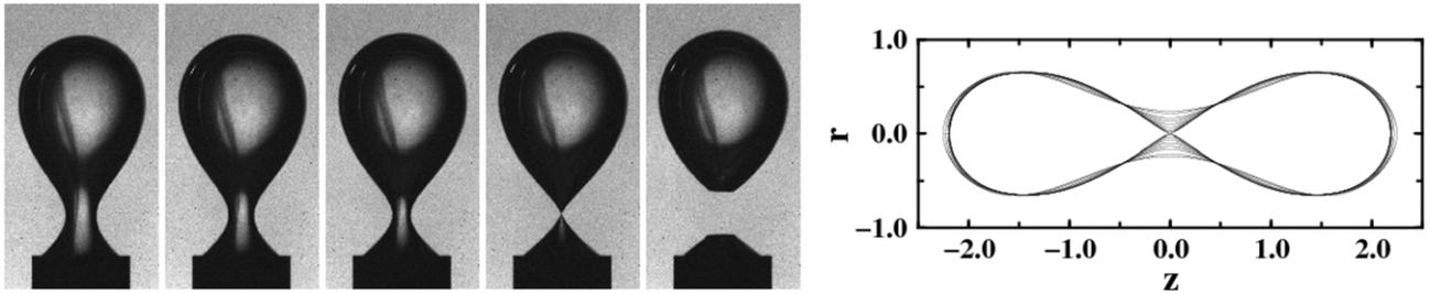
**Figure 55.** (Left) The pinch-off of an air bubble in water [326]. An initially smooth shape develops a localized pinch point. (Right) Numerical simulation of bubble pinch-off from initial conditions given by the shape with the largest waist; there is no gravity, so all shapes are symmetric about the pinch point. Reprinted with permission from [326], copyright 2007 by the American Physical Society.
