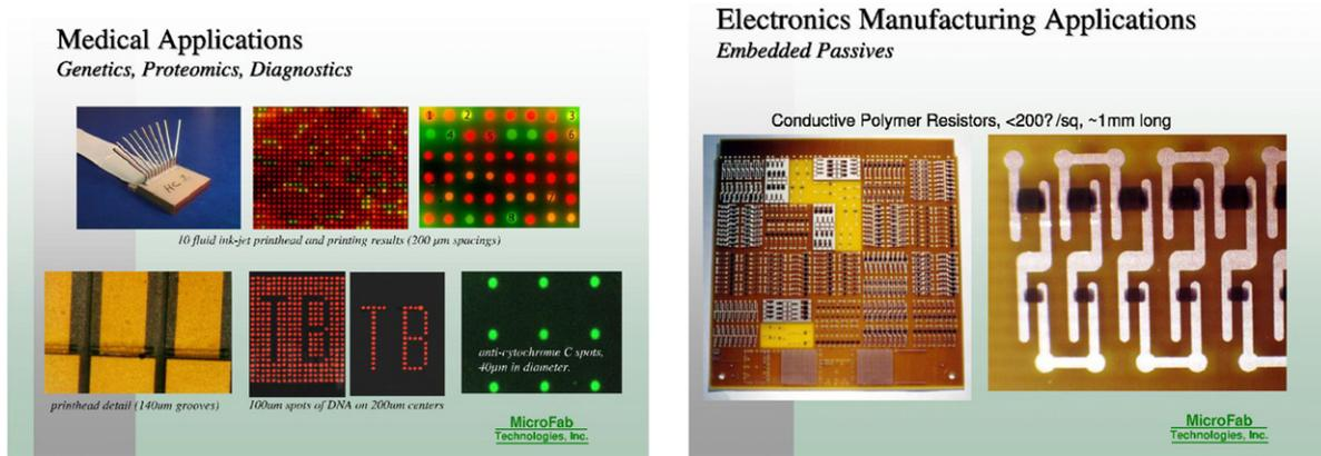
**Figure 63.** Commercial applications of ink-jet printing. The left panel shows so-called microarrays of drops laden with different biological samples. This permits one to test a large number of samples, using a small amount of space. The right panel shows integrated circuits, which can be printed ‘on-the-fly’ using ink jets.
