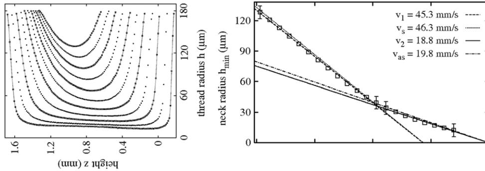
**Figure 53.** The neck of a falling drop of glycerol–water mixture [320],  $Oh = 0.49$ ,  $Bo = 0.047$ , making a transition from symmetric (Stokes) to asymmetric (NS) pinching. Accordingly, the rate of pinching changes at the transition point (right). The theoretical predictions for the two solutions are marked by the dotted and the dotted–dashed lines, respectively. Reprinted with permission from [320]. Copyright 2001 by the American Physical Society.
