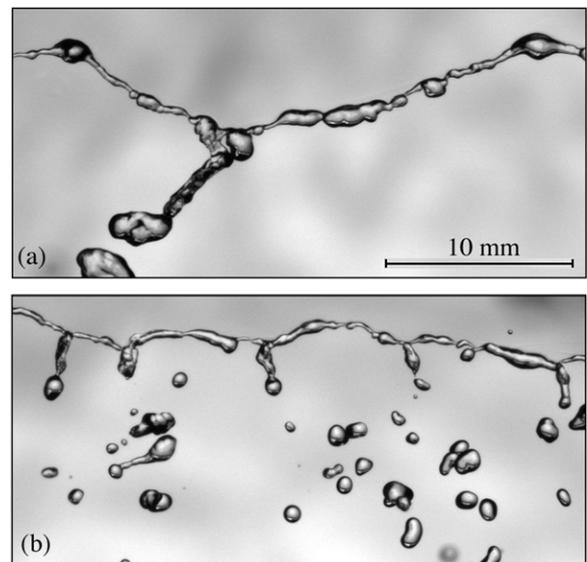
**Figure 78.** Close-up views of the free rim of a smooth liquid sheet, taken from the top (a). In (b), a periodic vibration of the impact point at 120 Hz has been added. The scale indicated in (a) is the same for both images, and  $h_0 = 3$  mm. Adapted from [278].
