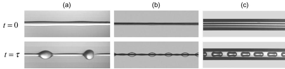
**Figure 24.** Capillary instability of cylindrical interfaces: (a) liquid jet, (b) liquid film on a fibre, (c) liquid film in a tube (adapted from [171]). The instability time  $\tau$  equals  $\sqrt{\rho h_0^3/\gamma}$  for a solid inviscid jet of radius  $h_0$ , and  $\eta h_0^4/(\gamma e_0^3)$  for a thin film of thickness  $e_0$  deposited on a fibre of radius  $h_0$ .
