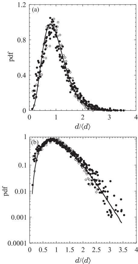
**Figure 93.** (a) Probability density functions of the drop size  $d$ , normalized by the arithmetic mean  $\langle d \rangle$ , for a number of jet velocities  $u_j$  and for several conditions of forcing  $\bullet$  as well as without forcing  $\circ$ . The solid curve represents the Gamma distribution with  $n = 5$ . (b) Semi-logarithmic representation of the size distributions shown in (a); for details see [278].
