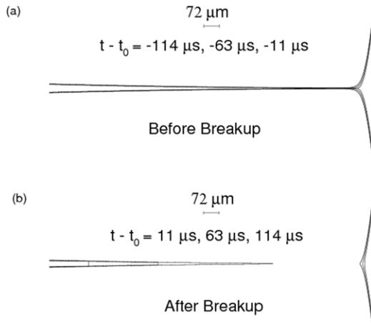
**Figure 62.** The breakup of a mixture of glycerol in four parts of ethanol, as calculated from similarity solutions before and after breakup. (a) shows three profiles before breakup, in time distances of  $46 \mu\text{s}$ , corresponding to  $|t'| = 1, 0.55$  and  $0.1$ . In part (b) the same is shown after breakup.
