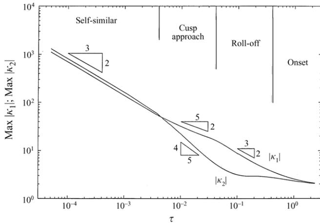
**Figure 88.** Time sequence of the maximum principal curvatures of a liquid bridge as it pinches-off under mild stretching (see also figure 87). Time  $\tau = t_p - t$  is the time from pinch-off. The onset of the instability, as well the boundary conditions influence the evolutions down to  $10^{-2}$ – $10^{-3}$  of the overall time  $t_p$ , after which the dynamics is universal. Adapted from [289].
