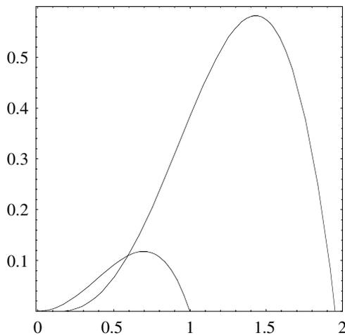
**Figure 41.** Stability curve  $-i\omega\tau$  versus  $kh_0$ . Destabilizing effect of surface charges with  $\Gamma = 2$  on the varicose mode  $m = 0$  in equation (150). The neutral jet dispersion curve is shown for comparison.
