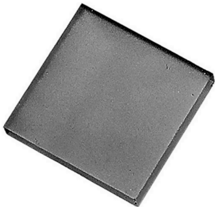
55477 LiF Crystal for Bragg Reflection
