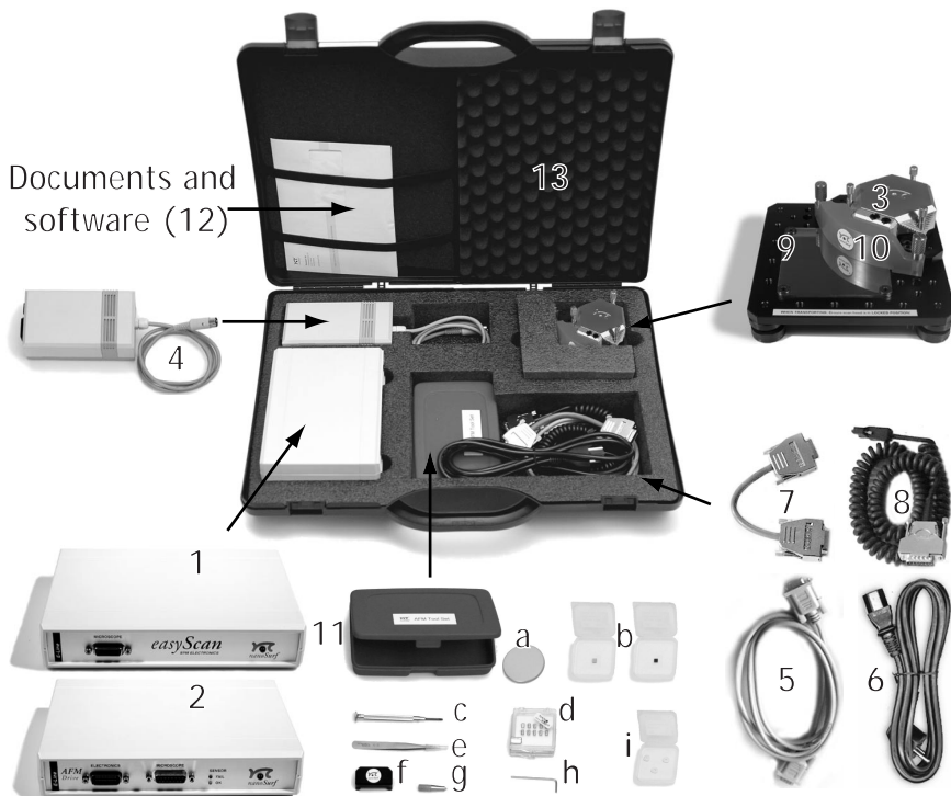
Components: The easyScan E-AFM system
