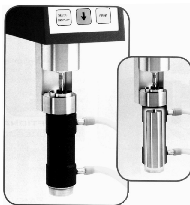
Figure 4. UL adapter consisting of a precision cylindrical spindle rotating inside an accurately machined tube to measure low viscosity accurately. It also has a water jacket to provide precise temperature control.
