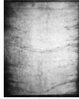
Figure 2. Image depicting liquid flow. In ER and MR fluids, the dipolar interaction is strong. If the field keeps on, the particles form chains along the field direction, which may jam the liquid flow.
