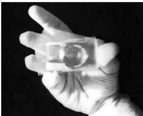
Near-normal reflection off a stack of microscope slides. You can see the image of the camera that took the picture. (E.H.)
