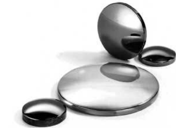
A group of semiconductor lenses made from ZnSe, CdTe, GaAs, and Ge. These materials are particularly useful in the infrared ( 2\ \mu\text{m} to 30\ \mu\text{m} ), where they are highly transparent despite the fact that they are quite opaque in the visible region of the spectrum. (Two-Six Incorporated/II-IV Inc.)
