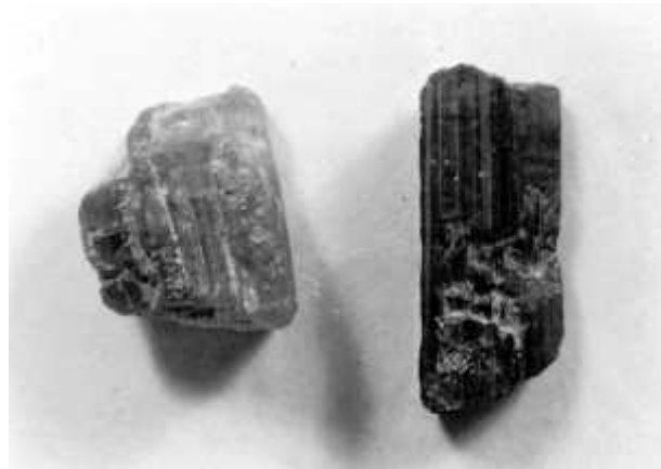
Figure 8.16 A dichroic crystal. The E -field parallel to the optic axis is transmitted without any diminution. The naturally occurring ridges evident in the photograph of the tourmaline crystals correspond to the optic axis. (E.H.)
