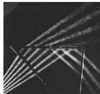
Figure 4.59 Internal reflection and the critical angle. (Educational Services, Inc.)
