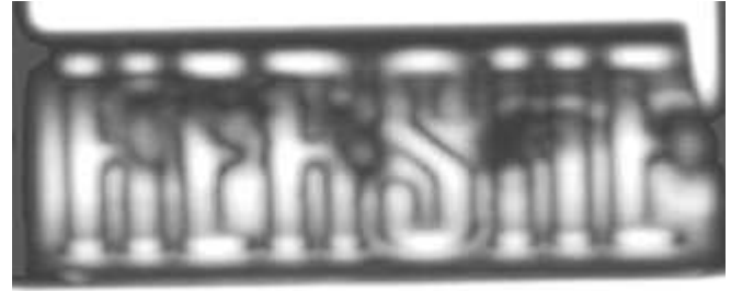
A picture of a candy bar made using T-rays. The nuts, which were hidden beneath the chocolate, are visible as a result of refraction. (V. Rudd, Picometrix, Inc.)
