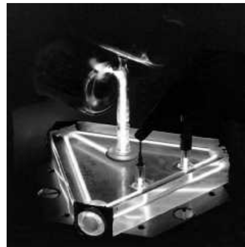
An early ring laser gyro. (Autonetics, a Division of Boeing North America, Inc.)
