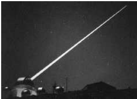
The creation of a laser guide star at the Phillips Laboratory, Kirtland Air Force Base, New Mexico. (Phillips Laboratory, Department of the US Air Force)
