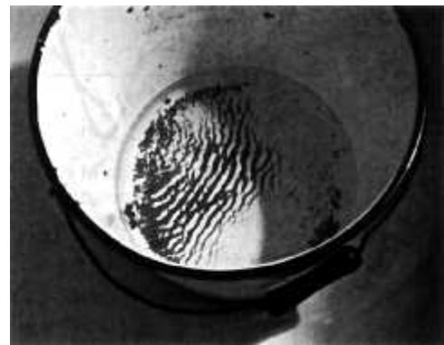
A pail used to wash a floor contained a suspension of fine dirt particles in water. When placed in a curved sink, the pail gently rocked along a fixed axis, setting up standing waves and distributing the particles in ridges as they settled. (E.H.)
