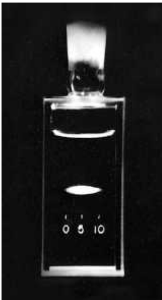
Figure 3.45 An ultrashort pulse of green light from a neodymium-doped glass laser. The pulse passed, from right to left, through a water cell whose wall is marked in millimeters. During the 10-picosecond exposure, the pulse moved about 2.2 mm. (Bell Laboratories)
