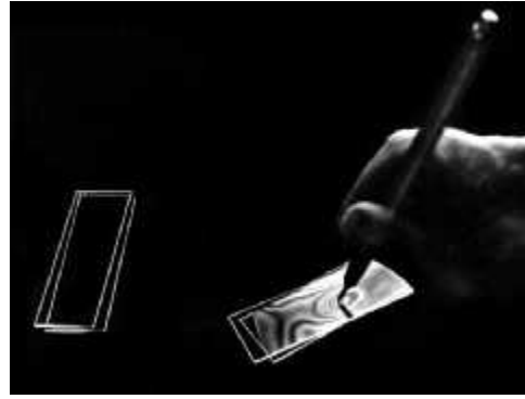
Fringes created by an air film between two microscope slides. (E.H.)
