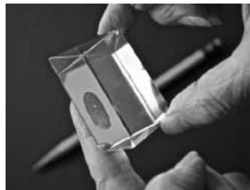
Frustrated total internal reflection on one face of a prism. (E.H.)
