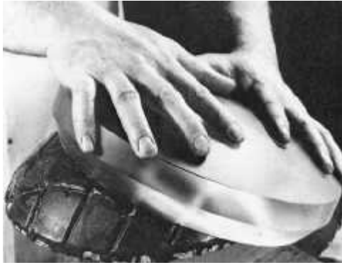
Polishing a spherical lens. (Optical Society of America)
