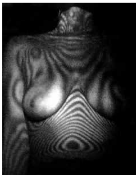
Double exposure holographic interferogram. (S. M. Zivi and G. H. Humberstone, "Chest motion visualized by holographic interferometry," Medical Research Eng. p. 5 [June 1970].) Compare this with the radar photo on page 451.
