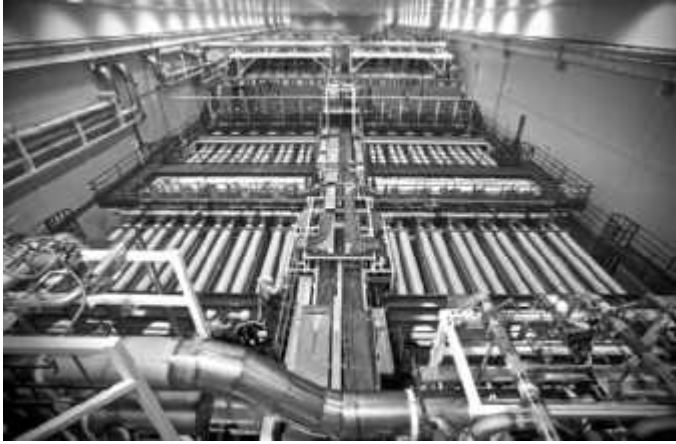
A portion of the NIF laser-based inertial confinement fusion device that essentially became operational in 2010. (Lawrence Livermore National Laboratory.)
