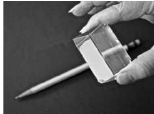
Total internal reflection on one face of a glass prism. (E.H.)
