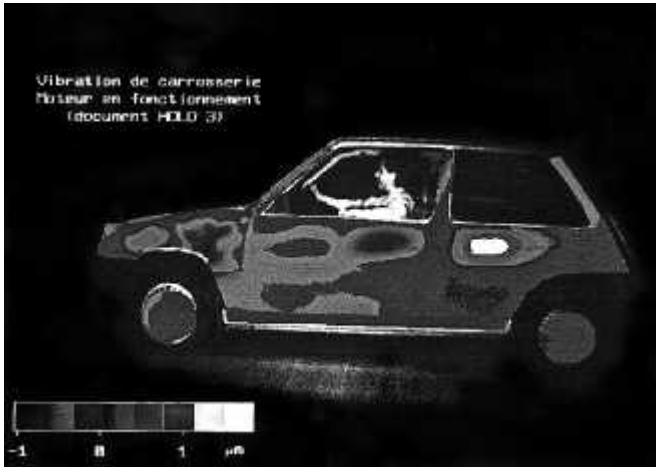
A standing-wave pattern on the side of a car due to vibrations caused by its running engine. The scale is in microns, where 1 \mu\text{m} = 10^{-6} \text{m} . The photo was made using a holographic technique. (HOL03/FTPO)
