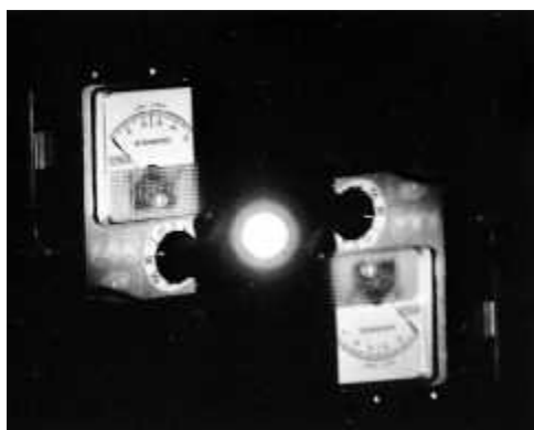
A reconstruction of a Fourier-transform hologram. (G.W. Stroke, D. Brumm, and A. Funkauser, J. Opt. Soc. Am. 55 , 1327 [1965].)
