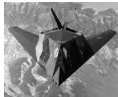
The F-117A Stealth fighter has an extremely small radar profile, that is, it returns very little of the incoming microwaves back to the station that sent them. That’s accomplished mostly by constructing the aircraft with flat tilted-planes that use the Law of Reflection to scatter the radar waves away from their source. One wants to avoid \theta_i = \theta_r \approx 0 . (US Dept of Defense)
