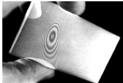
Newton's rings with two microscope slides. The thin film of air between the slides creates the interference pattern. (E.H.)
