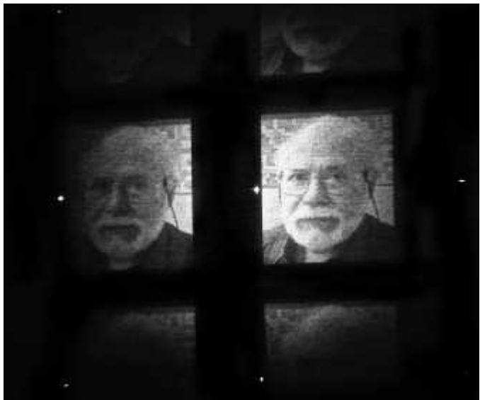
A hologram created using an LC-SLM. (Andreas Hermerschmidt and HOLOEYE Photonics AG, Berlin.)
