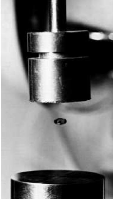
Ultrasonic levitation. Ultrasonic waves, one traveling up and the other down, form a standing-wave pattern. Here a droplet of water is suspended in a nodal region. (NASA)
