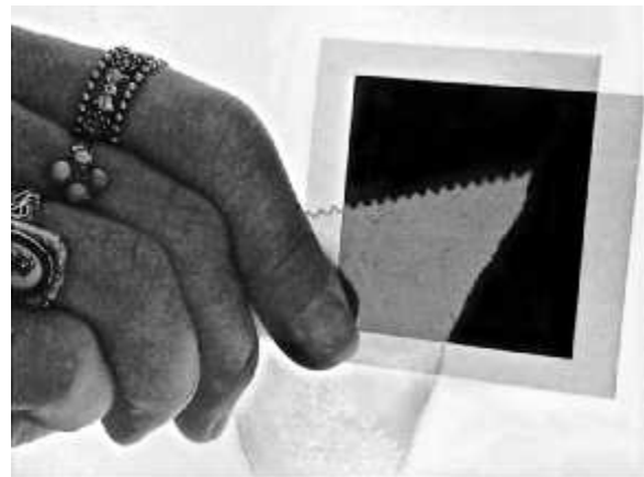
A piece of waxed paper between crossed polarizers. (E.H.)
