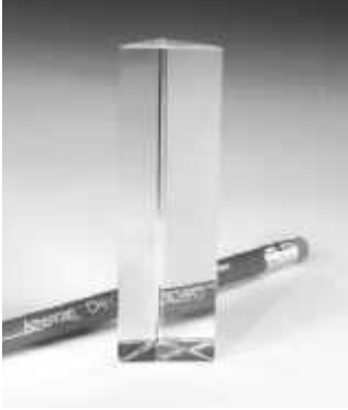
The prism behaves like a mirror and reflects a portion of the pencil (reversing the lettering on it). The operating process is total internal reflection. (E.H.)
