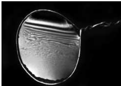
A wedge-shaped film made of liquid dishwashing soap. (E.H.)
