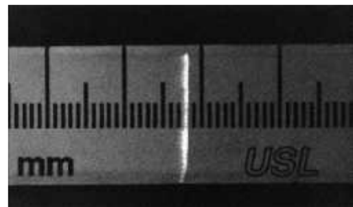
The image of a single collimated laser pulse caught as it swept along the surface of a ruler. This ultrashort burst of light corresponded to a portion of a plane wave. It extended in time for 300 \times 10^{-5} \text{ s} and was only a fraction of a millimeter long. (J. Valdmán and N. H. Abramson.)
