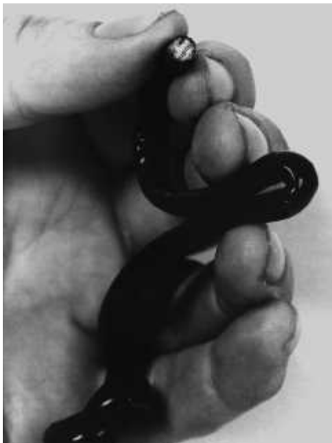
A coherent bundle of 10- \mu\text{m} glass fibers transmitting an image even though knotted and sharply bent. (American ACMI Div., American Hospital Supply Corp.)
