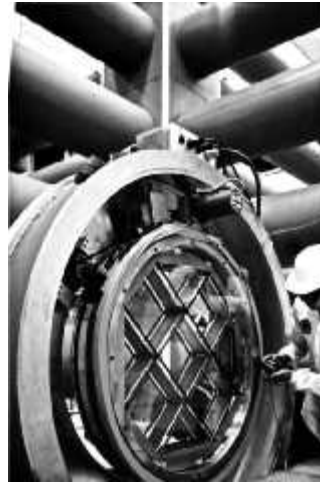
The KDP frequency converter for the Nova laser. (Lawrence Livermore National Laboratory.)
