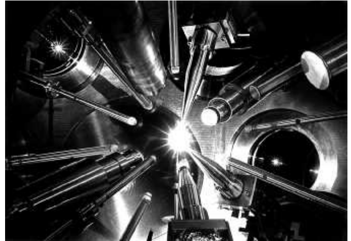
Inside the target chamber of the LLE laser-fusion device. Fusion reactions take place in tiny target-sphere filled with deuterium/tritium and irradiated by the 30-kJ Omega laser. (University of Rochester's Laboratory for Laser Energetic, Eugene Kowaluk, Image specialist.)
