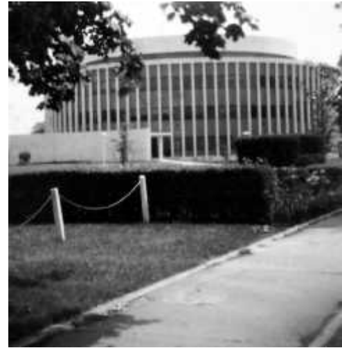
Photograph taken with a pinhole camera (Science Building, Adelphi University). Hole diameter 0.5 mm, film plane distance 24 cm, A.S.A. 3000, shutter speed 0.25 s. Note depth of field. (E.H.)
