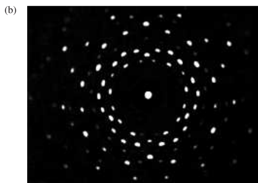
Figure 10.49 (a) Transmission Laue pattern. (b) X-ray diffraction pattern for quartz ( \text{SiO}_2 ). (E.H.)
