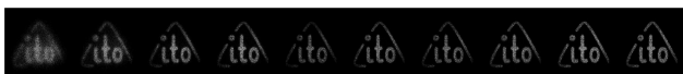
Fig. 11. Simulations of the effects of increasing sequential measurement distance (from left to right): \Delta z = 0.1 mm, \Delta z = 0.2 mm, . . . , \Delta z = 1 mm.
