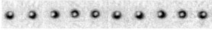
Fig. 23. – Phase-contrast images of a condensate being rotated at 1 Hz in a “doughnut” trap. The condensate (about 100\ \mu\text{m} in diameter) remains pierced by an off-resonant laser beam during its motion. Although angular momentum was clearly imparted to the cloud, we could not detect vortices. Figure taken from ref. [188].
