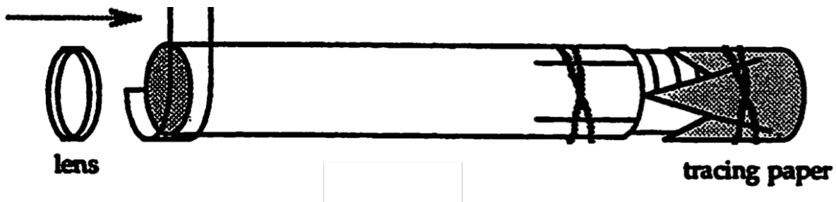
Figure 3: Replace the pinhole with the large lens using the red cap (not tape).
