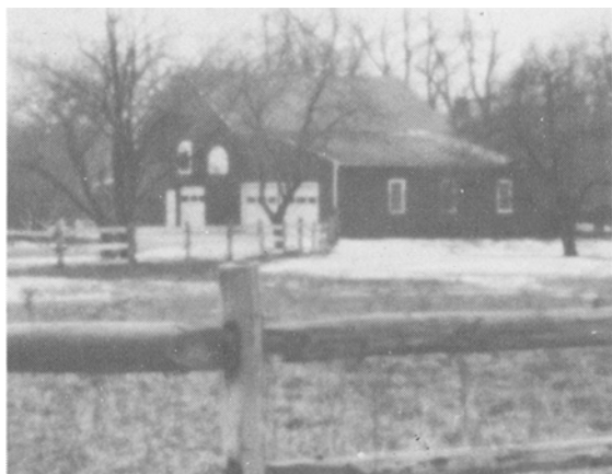
FIG. 9. Snapshot taken with pinhole camera to show characteristic soft focus and great depth of field.
