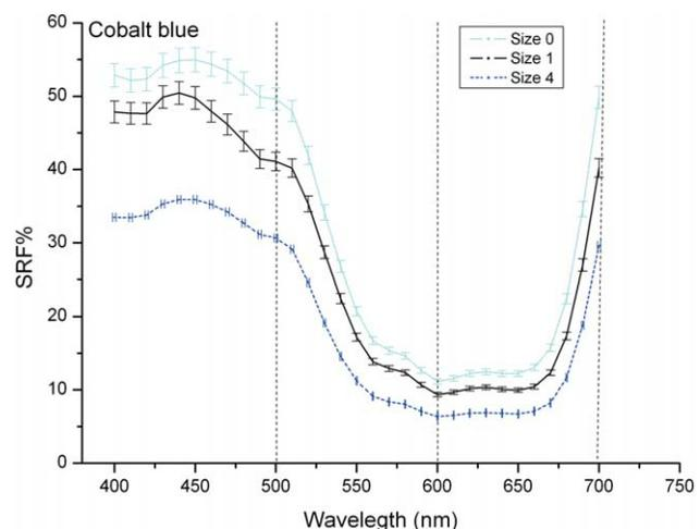
Fig. 5. Reflectance curve for the blue cobalt painting.
