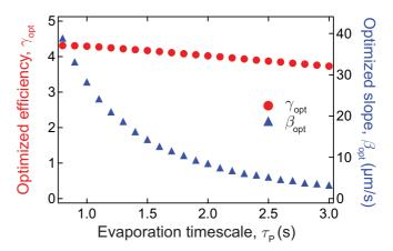
FIG. 4. CPM amplitude trajectory optimization for various power ramp time scales  $\tau_P$ . For each value  $\tau_P$  we run an optimization of the CPM reduction slope  $\beta$  (solid blue triangles) to maximize the evaporation efficiency  $\gamma$  (solid red circles) at  $\rho = 1$ .
