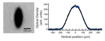
FIG. 7. Production of large, pure  $^{174}\mathrm{Yb}$  BECs using dynamical trap shaping to combat three-body inelastic loss. Absorption image (left) and horizontally integrated OD profile (right) after 50-ms ToF, with fit (solid line) to a Thomas-Fermi BEC density distribution, yielding a total of  $1.2\times10^6$  condensed atoms. The thermal fraction is consistent with zero.
