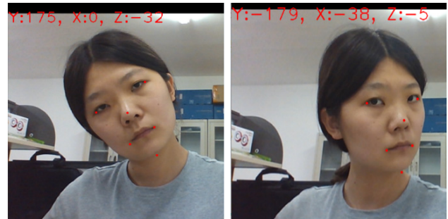
Fig. 7. Face attitude measurement result of front camera experiment.
