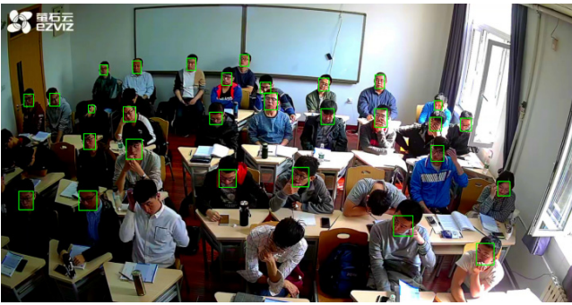
Fig. 4. The effect of face detection on MTCNN network under classroom.
