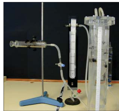
Fig. 1. The Cartesian diver is an inverted test tube with an air bubble trapped inside. The tube is placed in a closed 1-m long acrylic cylinder containing water. The pressure on the liquid surface in the cylinder is controlled with a syringe (on the left) and measured with a manometer (in the center).
