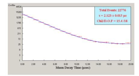
Once the muon lifetime is measured, a value of the Fermi coupling constant  $G_F$ , characterizing the strength of the weak interactions, is easily determined from the relation:
