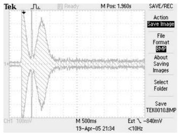
Figure 5: Pulsed Gradient Spin Echo
