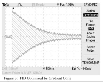
For this system to function correctly, the axis of the z-gradient  $(dB_z/dz)$  must lie along the axis of the local field. This is accomplished with the help of a sensitive dip compass inserted between the coil forms, at the place where the sample resides. The entire gradient coil assembly is then rotated about a horizontal axis until the local field is collinear with the z-axis of the coils. The coil assembly is then locked in place.
