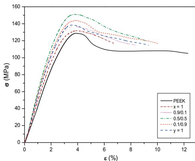
**Fig. 2.** Representative stress–strain curves at room temperature for the different PEEK based nanocomposites.
