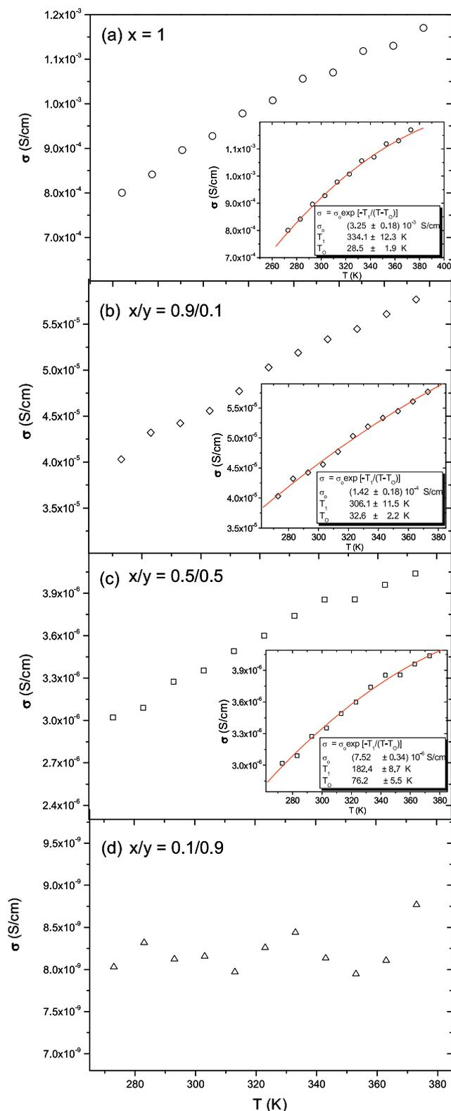
**Fig. 5.** Temperature dependence of the electrical conductivity of PEEK/SWCNT nanocomposite ( $x=1$ ) and PEEK/SWCNT/IF-WS<sub>2</sub> hybrid composites with different nanofiller contents. Note that PEEK and PEEK/IF-WS<sub>2</sub> ( $y=1$ ) are insulating materials ( $\sigma \sim 10^{-13}$  S cm<sup>-1</sup>), hence are not included in the plot.
