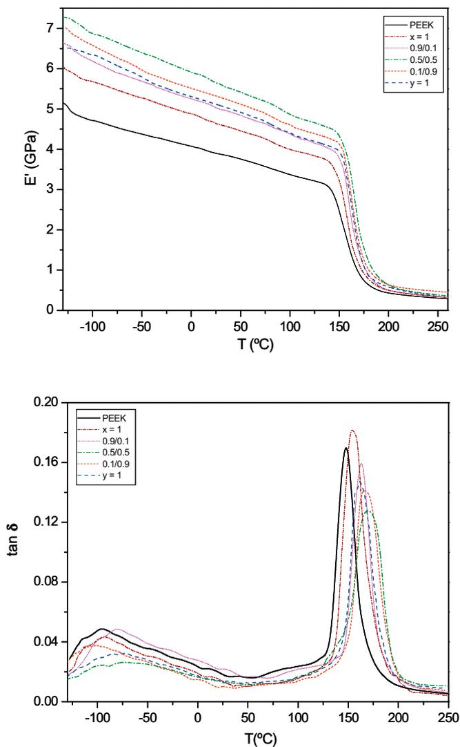
**Fig. 1.** Evolution of the storage modulus  $E'$  (a) and  $\tan \delta$  (b) as a function of temperature, at a frequency of 1 Hz, for PEEK and the hybrid nanocomposites incorporating different concentrations of SWCNTs and IF-WS<sub>2</sub>. For comparison, data of composites including a single type of filler are also included in the plot.
