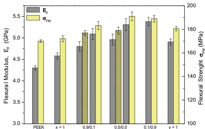
Fig. 3. Effect of SWCNTs and IF-WS<sub>2</sub> nanoparticles on the flexural modulus ( $E_F$ ) and flexural strength ( $\sigma_{FM}$ ) of PEEK at ambient temperature. The dashed bars correspond to samples prepared by a two-step melt-blending process.
