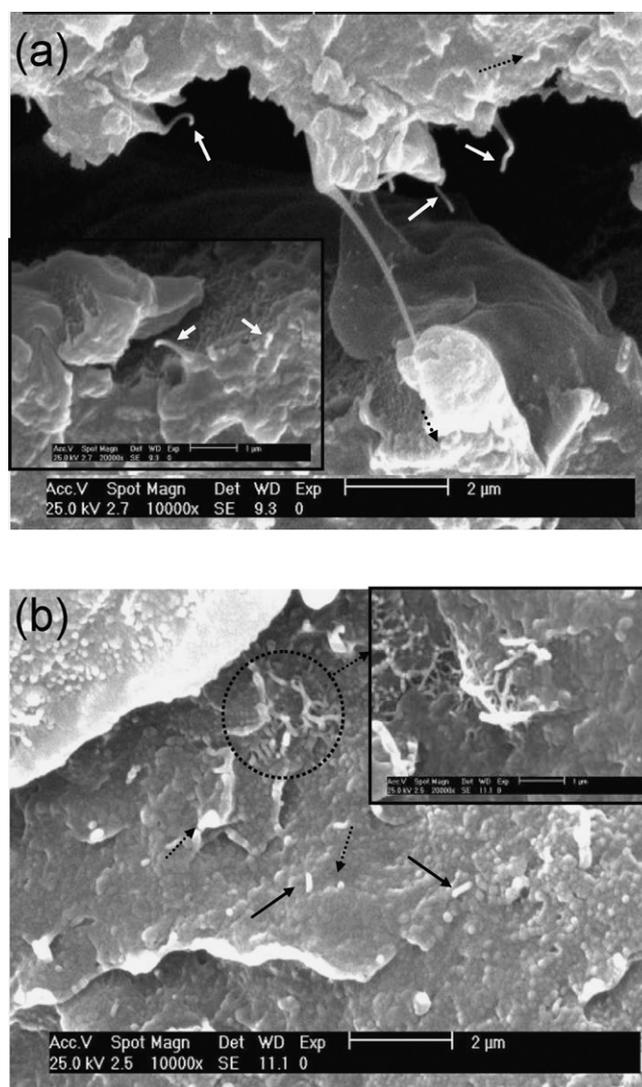
**Fig. 4.** Typical SEM micrographs from impact fractured surfaces of PEEK/SWCNT/IF-WS<sub>2</sub> ( $x/y=0.5/0.5$ ) hybrid nanocomposites prepared in a one-step process (a) and in two stages (b). The white arrows in (a) show SWCNTs pulled-out of the matrix. The black dashed and solid arrows in (b) point out nanoparticles and SWCNTs, respectively, randomly distributed through the PEEK matrix.
