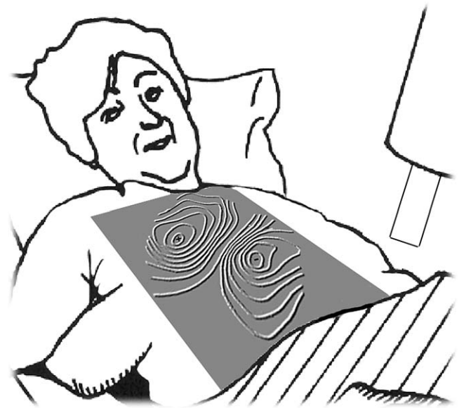
Fig. 4. Isofield map of magnetic flux density measured over a rectangular region of the thorax and abdomen.
