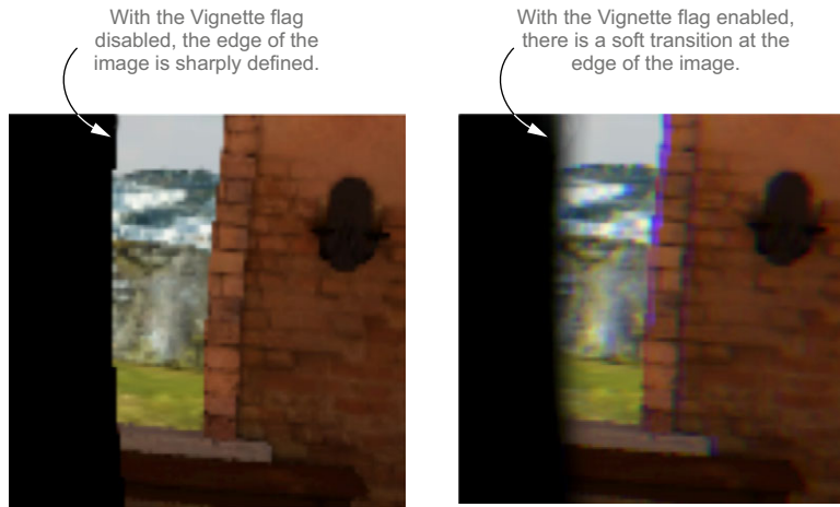
Figure 4.13 Comparison of the image edge with the vignette flag disabled (left) and enabled (right)
