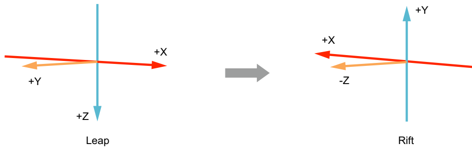
Figure 13.15 Transformation from Leap coordinates to Rift coordinates
